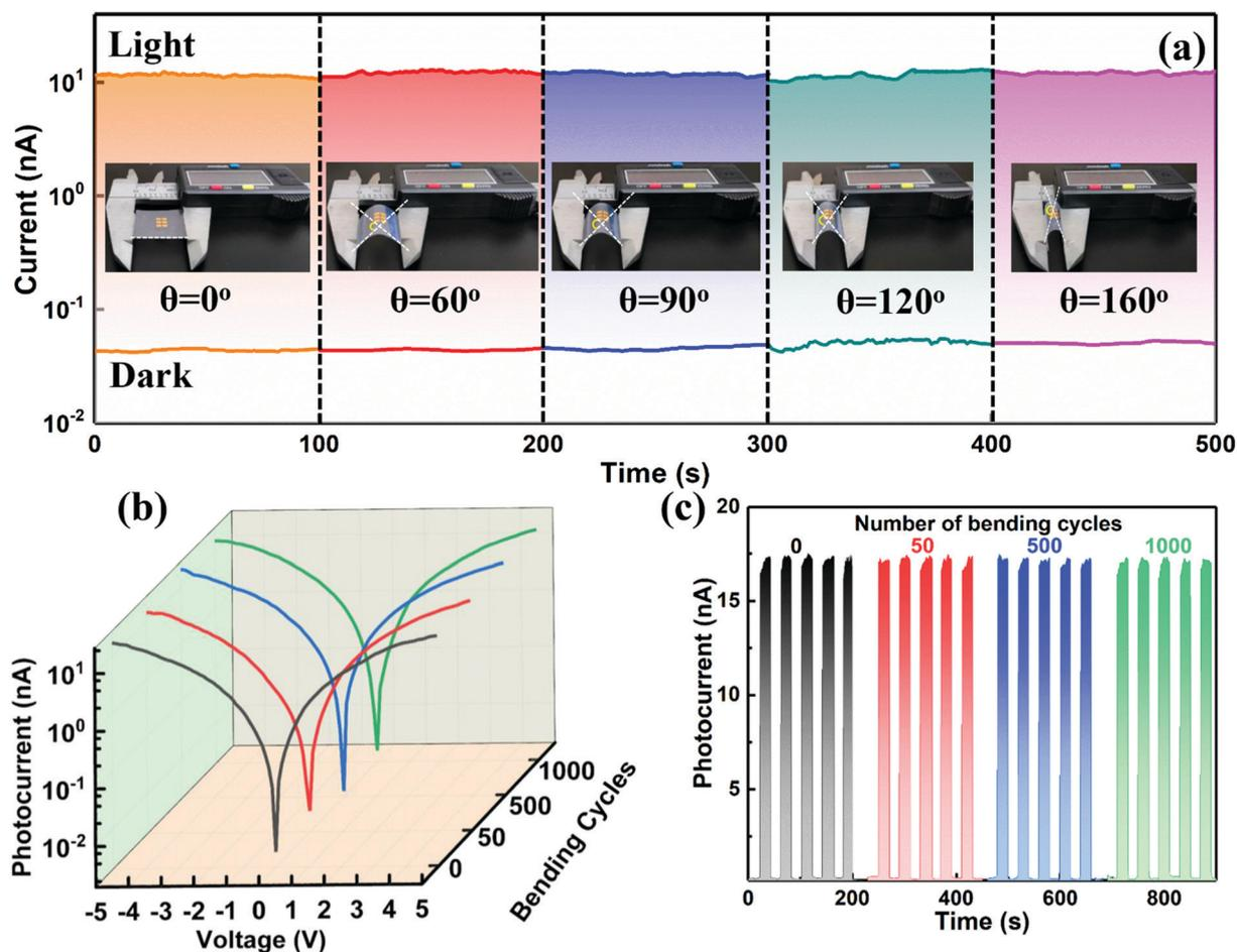
Fig. 4 (a) Output currents of the device with different bending angles under dark and light illumination with a light intensity of  $0.2 \text{ mW cm}^{-2}$  at a bias voltage of 5 V. The insets are the corresponding optical images of the device under five bending states.  $\theta$  is the bending angle. (b)  $I$ - $V$  and (c)  $I$ - $t$  curves of the device under different bending cycles.
