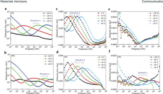
Fig. 3 Dependence of dielectric loss tangents of PS and FPS on frequency in a wide temperature range of -100 to 160 °C. (a and b) Dependence of dielectric loss and relaxations of PS (a) and FPS (b) at a high temperature range of 100-160 °C. (c and d) Dependence of dielectric loss and relaxations of PS (c) and FPS (d) at a mid-temperature range of 0-80 °C. (e and f) Dependence of dielectric loss and relaxations of PS (e) and FPS (f) at a low temperature range of -100 to -20 °C.
