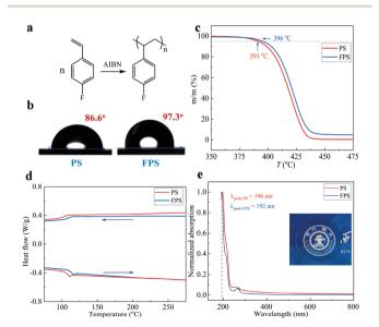
**Fig. 1** Chemical and physical characterization of FPS. (a) Synthesis of poly(4-fluorostyrene). (b) Water contact angles of PS ( $\theta=86.6^{\circ}$ ) and FPS ( $\theta=97.3^{\circ}$ ) films, respectively. (c) TGA profiles of PS and FPS. (d) DSC of PS and FPS. The arrows show the temperature scanning direction. (e) Normalized UV-vis absorption spectra of PS and FPS. Inset shows a photo of FPS coated glass (the circle shape in the photo) showing the high optical transparency of FPS.
