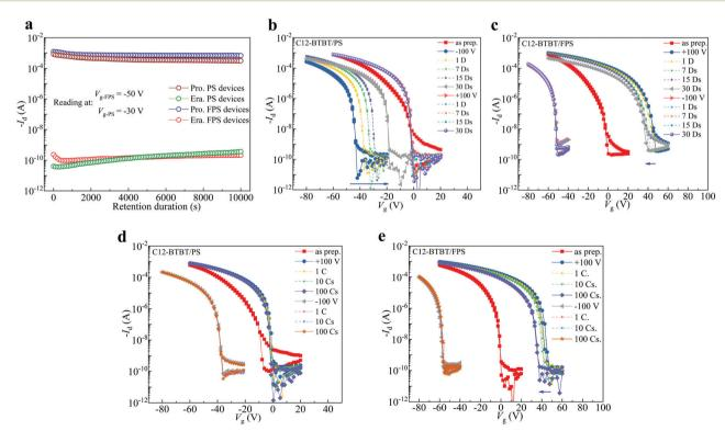
Fig. 5 Memory stability of C12-BTBT/PS and C12-BTBT/FPS OFET devices. (a) Retention characteristics of C12-BTBT/PS and C12-BTBT/FPS OFETs after programming and erasing. Ambient stabilities of C12-BTBT/PS (b) and C12-BTBT/FPS (c) OFETs with positive and negative electrets, D represents day. Repeatability over 100 cycles of C12-BTBT/PS (d) and C12-BTBT/FPS (e) OFETs with positive and negative electrets, C represents cycle.
