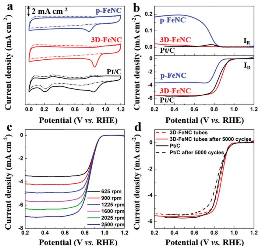
Fig. 5 (a) CV and (b) LSV curves of p-FeNC, 3D-FeNC, and Pt/C catalysts at 1600 rpm in  $N_2$  (dot line)/ $O_2$  (solid line)-saturated 0.1 M KOH solution. (c) LSV curves of the 3D-FeNC catalyst in  $O_2$ -saturated 0.1 M KOH solution at different rotating speeds. (d) LSV curves of the 3D-FeNC and Pt/C catalysts before and after 5000 cycles in  $O_2$ -saturated 0.1 M KOH solution at 1600 rpm. The scan rate is  $10 \text{ mV s}^{-1}$  for LSV curves in (b–d).
