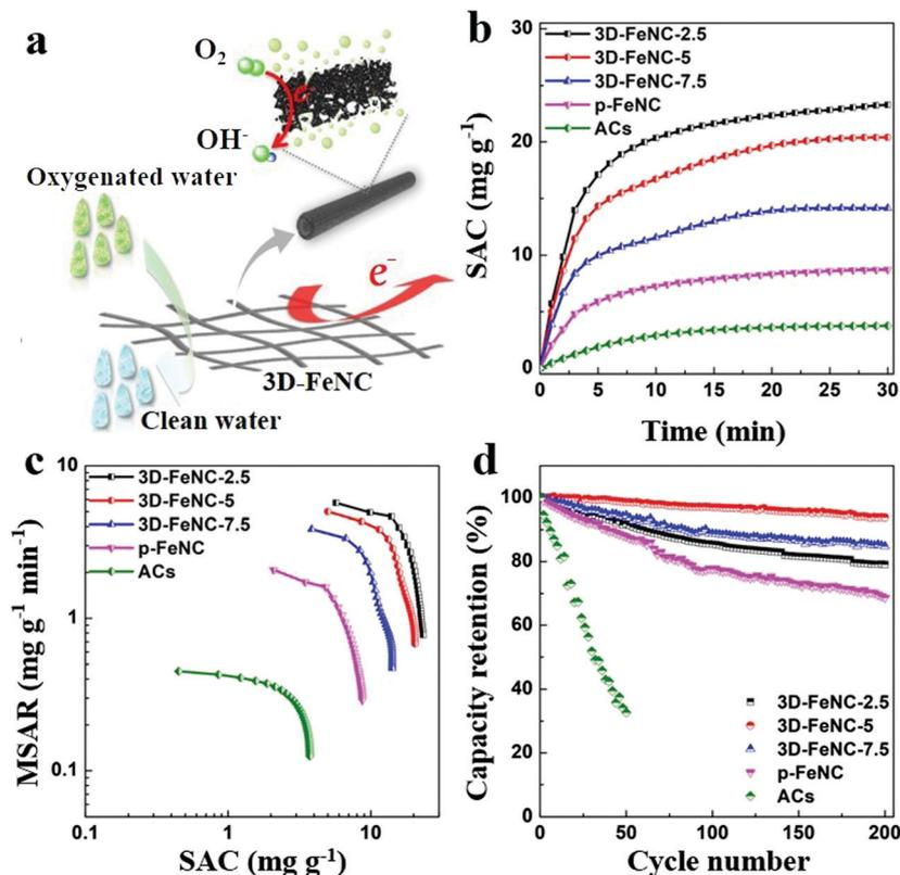
Fig. 6 (a) Schematic representation of the possible CDI process in oxygenated saline water using 3D-FeNC tubes. (b) SAC variations, (c) CDI Ragone plots, and (d) CDI cycling performances of 3D-FeNC- $y$  ( $y = 2.5, 5$  and  $7.5$ ), p-FeNC, and ACs in oxygenated saline water (5 mM).
