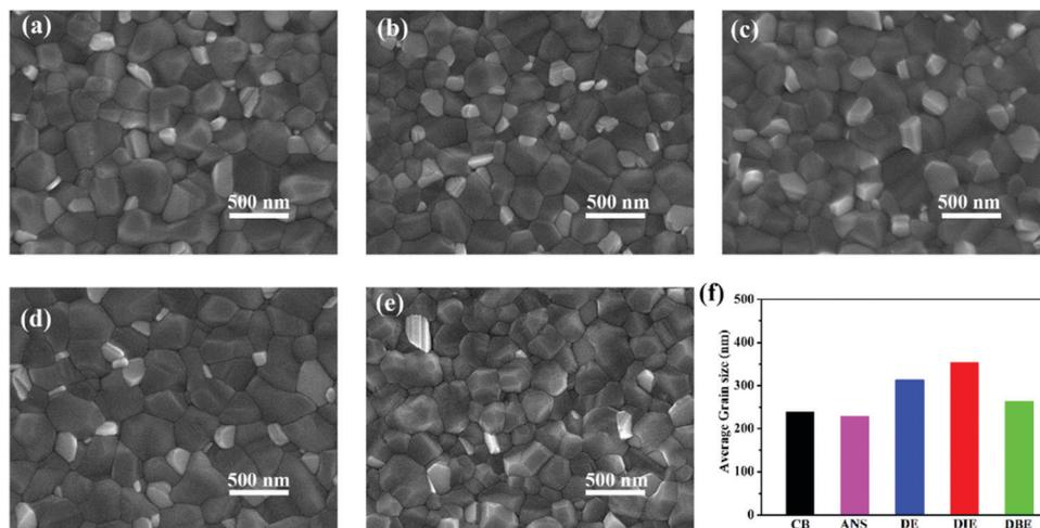
Fig. 2 (a–e) Top-view SEM images of the  $\text{Cs}_{0.05}(\text{MA}_{0.17}\text{FA}_{0.83})\text{Pb}(\text{I}_{0.83}\text{Br}_{0.17})_3$  films prepared using (a) CB, (b) ANS, (c) DE, (d) DE, and (e) DBE as antisolvents. (f) Average grain sizes of the  $\text{Cs}_{0.05}(\text{MA}_{0.17}\text{FA}_{0.83})\text{Pb}(\text{I}_{0.83}\text{Br}_{0.17})_3$  films prepared using the various antisolvents.
