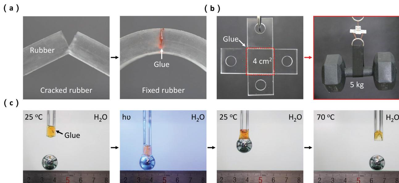
**Fig. 5** Applications of 9-anth-PEI glue. (a) Precise adhesion of 9-anth-PEI glue on cracked silicone rubber surfaces after irradiation for 2 min. (b) An underwater adhered sample holding 5 kg of weight with a 4 cm<sup>2</sup> adhesive area. (c) Controllable underwater transport process of a steel ball using 9-anth-PEI glue.
