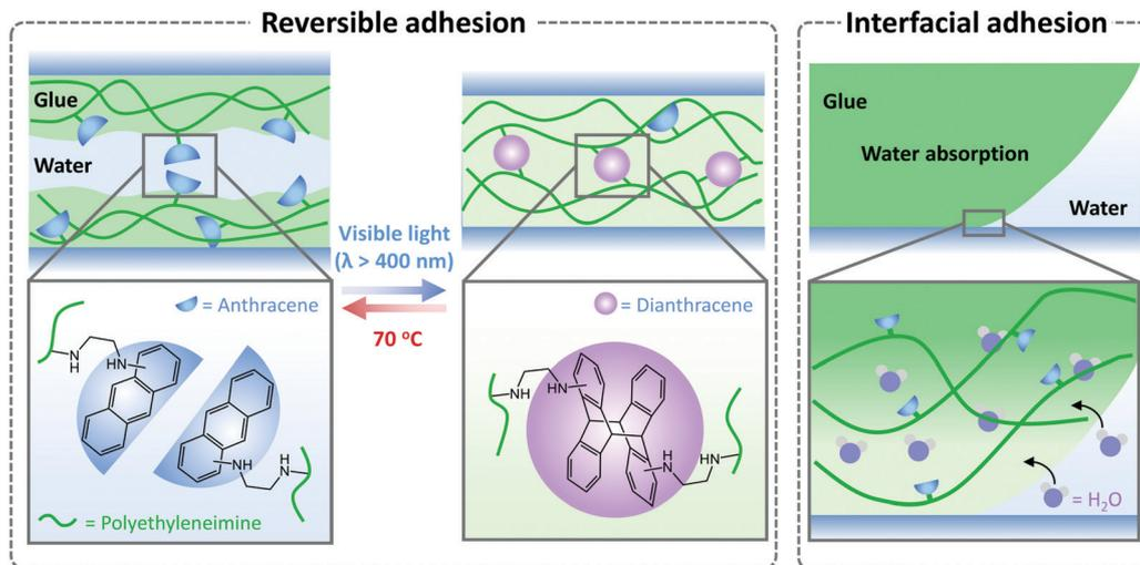
**Fig. 1** Design of the anthracenyl-functionalized polyethyleneimine (anth-PEI) as a reversible underwater glue. Due to the reversible crosslinking of anth-PEI networks, the glue can achieve switchable underwater adhesion under orthogonal physical stimuli. The hygroscopic and hydrophilic anth-PEI glue can spontaneously spread over the surfaces and absorb interfacial water, achieving effective interfacial adhesion.
