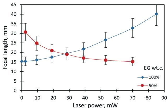
Fig. 4 The focal length of the liquid lenses (1  $\mu\text{l}$  in volume) of pure ethylene glycol and its 50% mixture with ethyl alcohol vs. the power of the laser beam.
