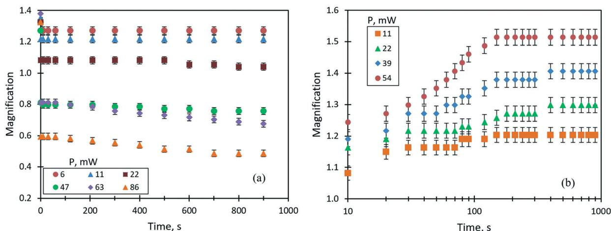
Fig. 8 Evolution of the linear magnification of liquid lenses at different powers of the laser beam: (a) benzyl alcohol (0.6  $\mu\text{l}$ ), the thermocapillary mechanism; (b) 50% mixture of ethylene glycol and ethyl alcohol (1  $\mu\text{l}$ ), the solutocapillary mechanism.
