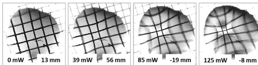
Fig. 7 Images of the test grid obtained with the thermocapillary lens (benzyl alcohol, 0.6  $\mu\text{l}$ ) at different laser beam powers.<sup>30</sup>
