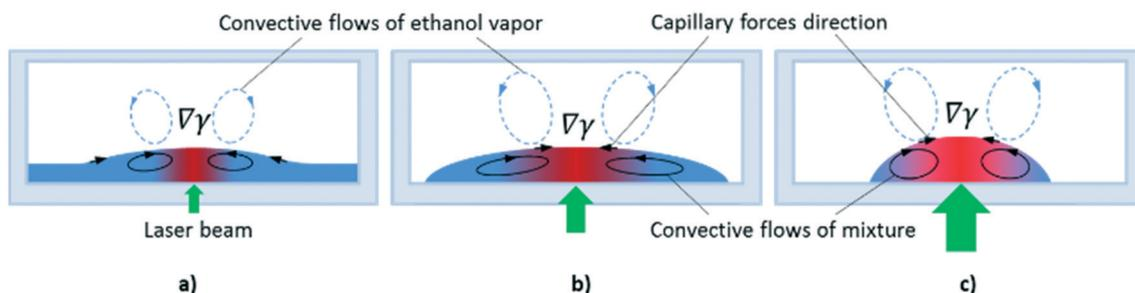
Fig. 3 Schema of the droplet formation process in a layer of liquid mixture induced by the laser beam.  $\nabla\gamma$  is the concentration surface tension gradient along the interface. (a) The convex deformation of the layer caused by the laser beam; (b) formation of the droplet in the layer; (c) the droplet shrinkage caused by the laser power increasing.
