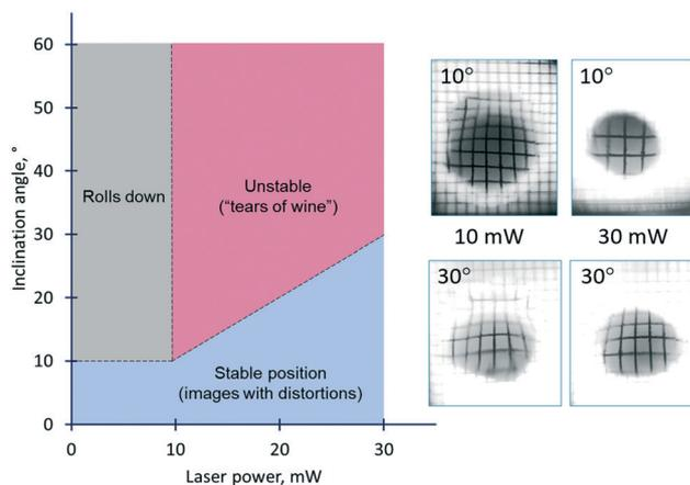
**Fig. 10** The stability diagram of the solutocapillary lens (50% mixture of ethylene glycol and ethyl alcohol, 1  $\mu\text{l}$ ) operating at different angles of inclination (0–60°) and powers of the laser beam. The borders (dashed lines) between areas in the diagram are drawn approximately. On the right – the images of the test grid for the different tilt angles of the lens and laser beam powers.
