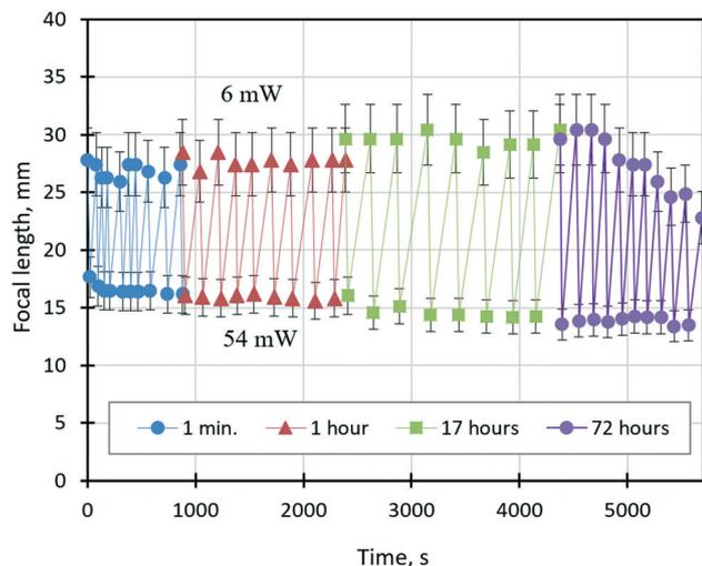
**Fig. 9** The dependence of the focal length of the solutocapillary lens (50% mixture of ethylene glycol and ethyl alcohol, 1  $\mu\text{l}$ ) on the cyclically (10 times for a series) changing power of the laser beam between 6 mW (the upper symbols) and 54 mW (the lower symbols). The time intervals between series when the laser beam is off: 1, 17 and 72 hours. The experiment started in 1 minute after the liquid was deposited in the cell.
