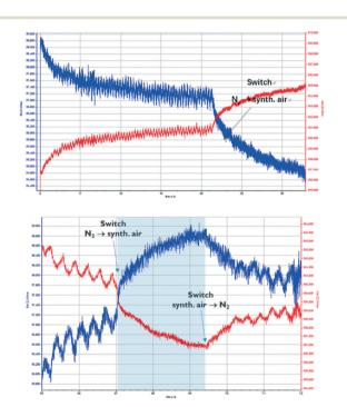
Fig. 6 The effect of diluting gas on the impedance of Zn-MOF-74 measured in N2 and synthetic air by exposure to CO2 concentration that alternates between 0 and 1000 ppm every 10 minutes (top) and the reversibility of the deactivation of the Zn-MOF-74-based sensor upon exposure to oxygen in synthetic air (bottom).
