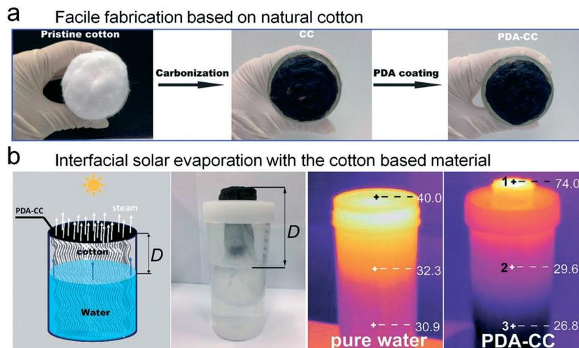
Fig. 12 Low-cost cotton based solar evaporator. (a) The rapid fabrication of light absorbing cotton. (b) The oil lamp inspired solar evaporator exhibits an obvious interfacial heating ability.<sup>70</sup>
