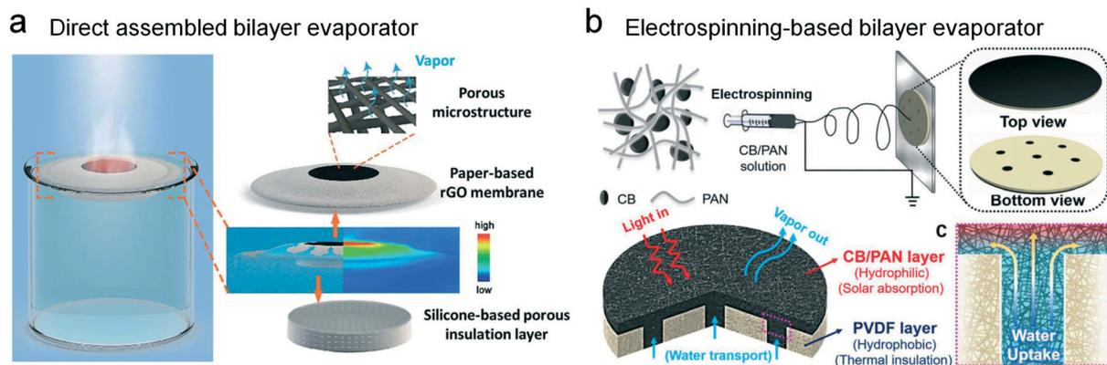
Fig. 6 Integrated solar evaporators with an external floating apparatus. (a) The silicone-based insulation layer as a supporting substrate for the graphene membrane.<sup>48</sup> (b) The PVDF substrate acting as the floater to support the electrospun light-absorbing fabric.<sup>49</sup> (c) The water channel.
