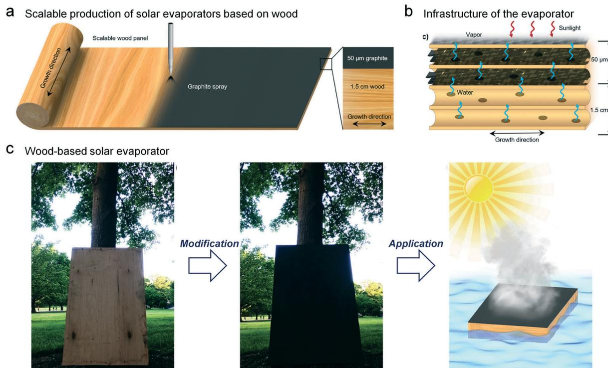
Fig. 13 Low-cost and scalable wood-based solar evaporator.<sup>71</sup> (a) The fabrication of the wood-based light-absorbing material via a graphite spraying method. The thickness of the light-absorbing layer is 50 μm and that of the insulating layer is about 1.5 cm. (b) The water can transfer to the evaporation interface through the wood lumens. (c) The demonstration of scalable fabrication and the application of the wood-based floatable evaporator.
