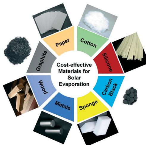
**Fig. 11** The cost-efficient materials that are used in solar evaporation, including low price photothermal materials (carbon black and graphite), cellulose-based hydrophilic substrates (paper and cotton), and effective floating supports (wood and sponge).
