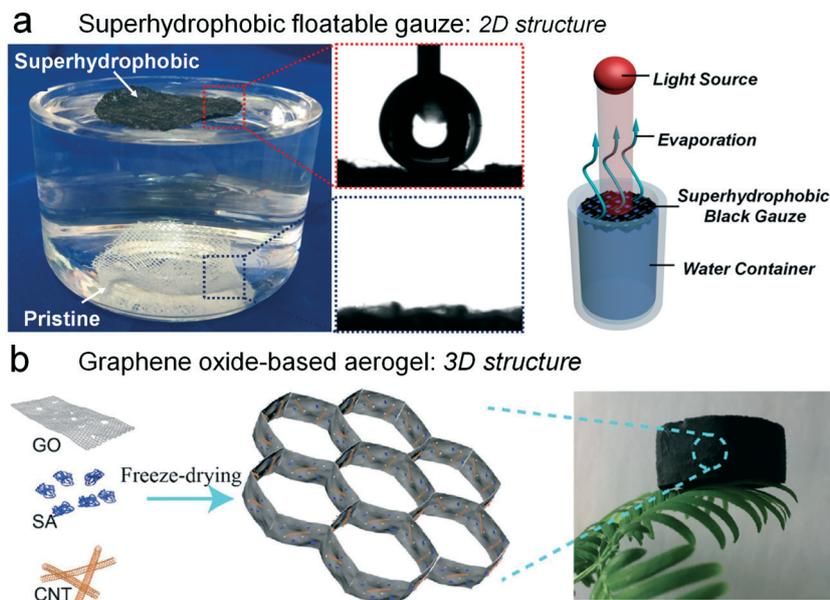
**Fig. 5** Intrinsic floatable solar evaporators. (a) The carbon black-based, self-cleaning, superhydrophobic gauze for efficient solar evaporation at the air–water interface.<sup>45</sup> (b) The graphene oxide-based aerogel with ultralow density for solar steam generation.<sup>47</sup>
