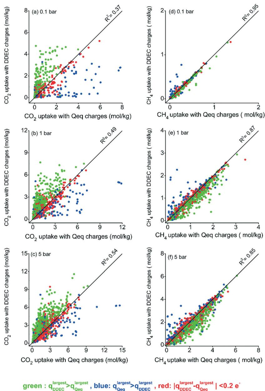
Fig. 1 CO<sub>2</sub> uptakes (a–c) and CH<sub>4</sub> uptakes (d–f) obtained from simulations using Qeq and DDEC charges at 0.1, 1, and 5 bar for the 10/90 CO<sub>2</sub>/CH<sub>4</sub> mixture.
