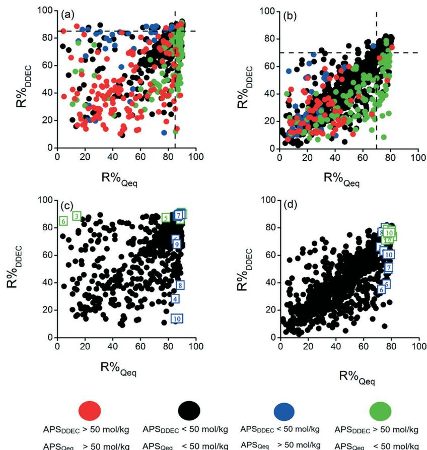
**Fig. 3** Comparison of R% of DDEC and Qeq-charged MOFs under (a and c) VSA (b and d) PSA conditions for the 10/90 CO<sub>2</sub>/CH<sub>4</sub> mixture. Dashed lines show R% = 85% in (a) and R% = 70% in (b). The top 10 MOFs identified by DDEC and Qeq methods are shown in green and blue, respectively.
