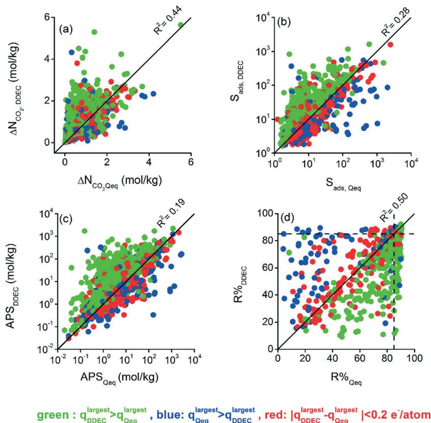
**Fig. 2** Calculated adsorbent performance evaluation metrics using Qeq and DDEC charges under VSA conditions at 298 K, for the 10/90 CO<sub>2</sub>/CH<sub>4</sub> mixture; (a)  $\Delta N_{\text{CO}_2}$ , (b)  $S_{\text{ads}}$ , (c) APS, and (d)  $R\%$ . Dashed lines in (d) show  $R\% = 85\%$ .
