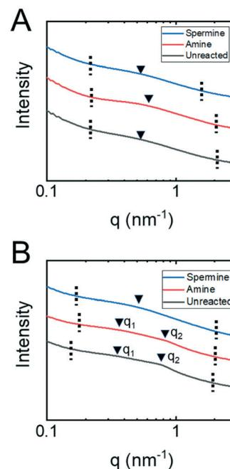
**Fig. 4** One-dimensional SAXS traces for P(TFEMA-OEGMA-GMA) copolymer membranes (A) in the dry state and (B) submerged in water. The dashed vertical lines indicate the region of interest and the arrows identify maxima in the broad scattering peaks. The scaling and positions of the traces on the y-axis have been altered to facilitate visualizing the peak positions in reference to  $q$ -values.
