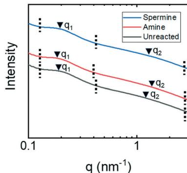
Fig. 7 One-dimensional SAXS traces for P(TFEMA-OEGMA-GMA) copolymer membranes submerged in ethanol. The dashed vertical lines indicate the region of interest and the arrows identify maxima in the broad scattering peaks. The scaling and positions of the traces on the y-axis have been altered to facilitate visualizing the peak positions in reference to  $q$ -values.
