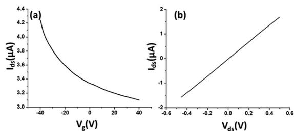
**Fig. 2** (a) Field-effect characteristics of rGO was tested with a back-gate voltage from -40 to 40 V, with a 0.1 V bias voltage loaded between the source and the drain electrodes. The identified current on/off ratio is ~1.4. (b)  $I$ - $V$  characterization of rGO with the source drain voltage from -0.5 to 0.5 V.
