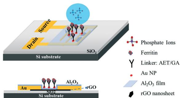
**Fig. 1** Schematic diagram and side view of the rGO-based FET device for phosphate ion detection. The gaps between the interdigitated Au electrodes are bridged by single-layer rGO nanosheets. The sensing area is covered by a thin Al<sub>2</sub>O<sub>3</sub> film (~4 nm) with surface-deposited Au NPs (~4 nm diameter). The ferritin probes were immobilized on Au NPs with an AET/GA linker.
