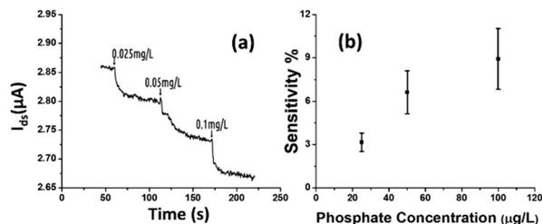
**Fig. 6** (a) Dynamic responses of the rGO-FET sensor to phosphate ions with concentrations of 25  $\mu\text{g L}^{-1}$ , 50  $\mu\text{g L}^{-1}$ , and 100  $\mu\text{g L}^{-1}$ . (b) The relationship between the phosphate concentration and the corresponding sensitivity shown by the sensing platform. The lower detection limit could reach down to 10  $\mu\text{g L}^{-1}$ .
