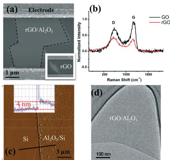
**Fig. 3** (a) SEM image of the Al<sub>2</sub>O<sub>3</sub> film covering the rGO sheet. Inset: rGO sheet spans across the interdigitated electrode gap and is transparent under the electron beam. (b) Raman spectra of GO (black) and rGO (red). (c) AFM image of the Al<sub>2</sub>O<sub>3</sub> film; the solid black line indicates the scanning trace; inset: height profile. (d) TEM image of the Al<sub>2</sub>O<sub>3</sub> film covering the rGO nanosheet.
