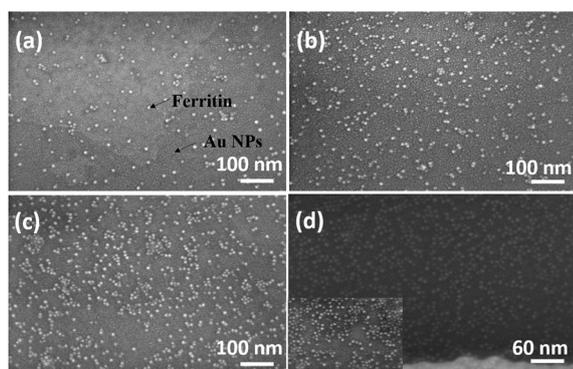
**Fig. 4** SEM images of immobilized ferritin with a ferritin concentration of 5 mg mL<sup>-1</sup> at pH values of (a) 7.83, (b) 6.98, (c) 5.10, and (d) 4.26.
