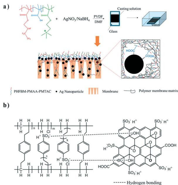
**Fig. 4** a) Fabrication process and structure of a PVDF/Ag/PHFBM-PMAA-PMTAC membrane. b) Schematic illustration of the interactions within an interpenetrating network/SGO composite membrane. Reproduced with permission from ref. 52 and 53. Copyright 2019 and 2018, Elsevier.
