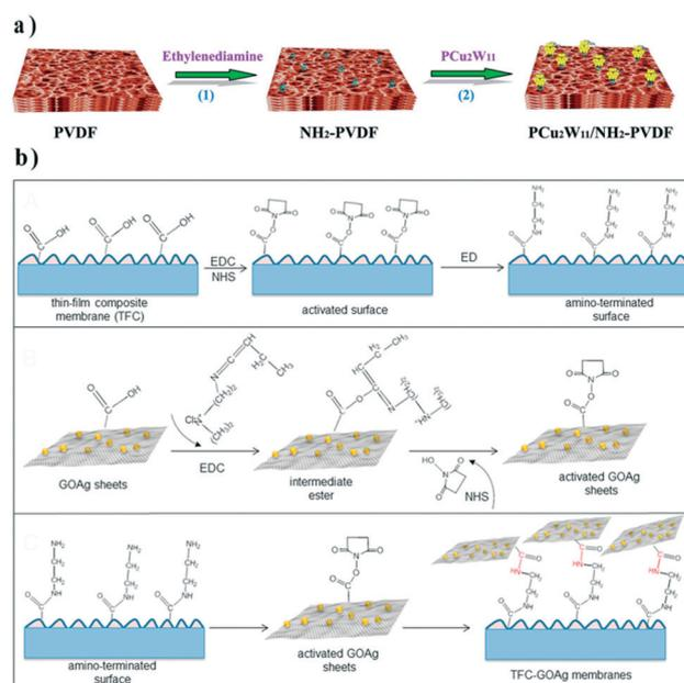
Fig. 5 Fabrication process of a) the  $\text{PCu}_2\text{W}_{11}/\text{NH}_2\text{-PVDF}$  interface composite membrane and b) binding GO–Ag nanosheets on the TFC membrane. Reproduced with permission from ref. 66 and 67. Copyright 2017, Elsevier.
