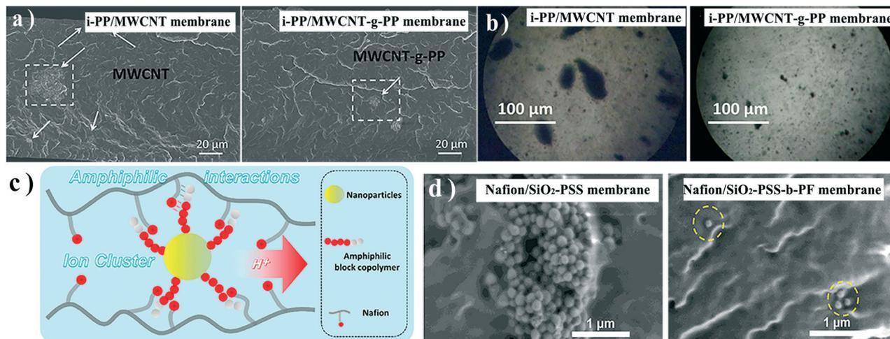
**Fig. 2** a) Cross-sectional SEM images and b) optical micrographs of the i-PP/MWCNT membrane and i-PP/MWCNT-g-PP membrane. c) Schematic illustration of the interaction between Nafion and amphiphilic block copolymer grafted nanoparticles. d) Cross-sectional SEM images of Nafion/SiO<sub>2</sub>-PSS and Nafion/SiO<sub>2</sub>-PSS-b-PF membranes. Reproduced with permission from ref. 36 and 38. Copyright 2017 and 2018, Elsevier.
