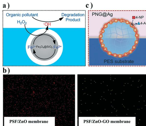
**Fig. 3** a) Schematic illustration of Fe<sub>3</sub>O<sub>4</sub>@SiO<sub>2</sub> NPs in a membrane; b) FESEM mapping images of PSF/ZnO and PSF/ZnO-GO membranes and c) schematic illustration of the Ag-loaded nanogel at the membrane/feed interface. Reproduced with permission from ref. 44–46. Copyright 2019 and 2017, Elsevier; Copyright 2018, Wiley-VCH Verlag GmbH & Co. KGaA.
