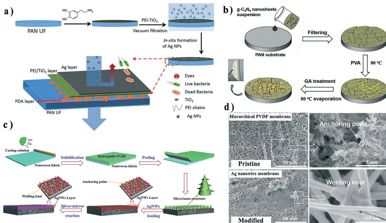
**Fig. 8** Fabrication process of a) the PEI-TiO<sub>2</sub>/Ag composite PAN membrane, b) g-C<sub>3</sub>N<sub>4</sub> nanosheet dual-layer composite membrane, and c) Ag nanowire dual-layer composite membrane. d) SEM images of pristine hierarchical PVDF membrane and Ag nanowire membrane surfaces after the silver-mirror reaction. Reproduced with permission from ref. 92, 93 and 96. Copyright 2019, Elsevier; Copyright 2018, Wiley-VCH Verlag GmbH & Co. KGaA.
