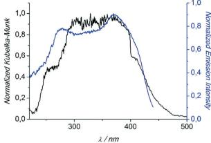
Fig. 6 Diffuse reflectance (black) and excitation (blue) spectra of 1. The excitation spectrum was monitored at 540 nm. Both spectra are normalized to allow comparison.
