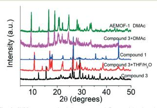
Fig. 4 PXRD patterns of pristine compound 3, materials after the treatment of compound 3 with THF/ $H_2O$  and DMAc  $\emph{vs.}$  those of compound 1 and AEMOF-1-DMAc.
