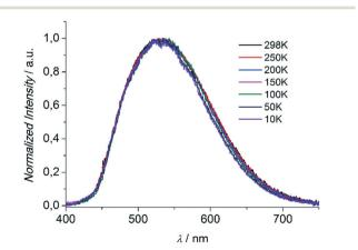
Fig. 7 Solid state fluorescence spectra of compound 1 at different temperatures upon excitation at 350 nm.
