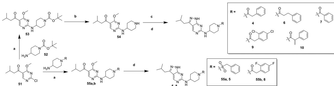
**Scheme 1** Synthesis of compounds 4–10. (a) *N,N*-Diisopropylethylamine (DIPEA), butan-1-ol; (b) trifluoroacetic acid (TFA), dichloromethane (DCM), 97% (over 2 steps); (c) *R*-COOH, *N,N,N',N'*-tetramethyl-*O*-(benzotriazol-1-yl)uronium tetrafluoroborate (TBTU), DIPEA, DCM; (d) hydrazine hydrate, butan-1-ol, 30–56% (over 2 steps).
