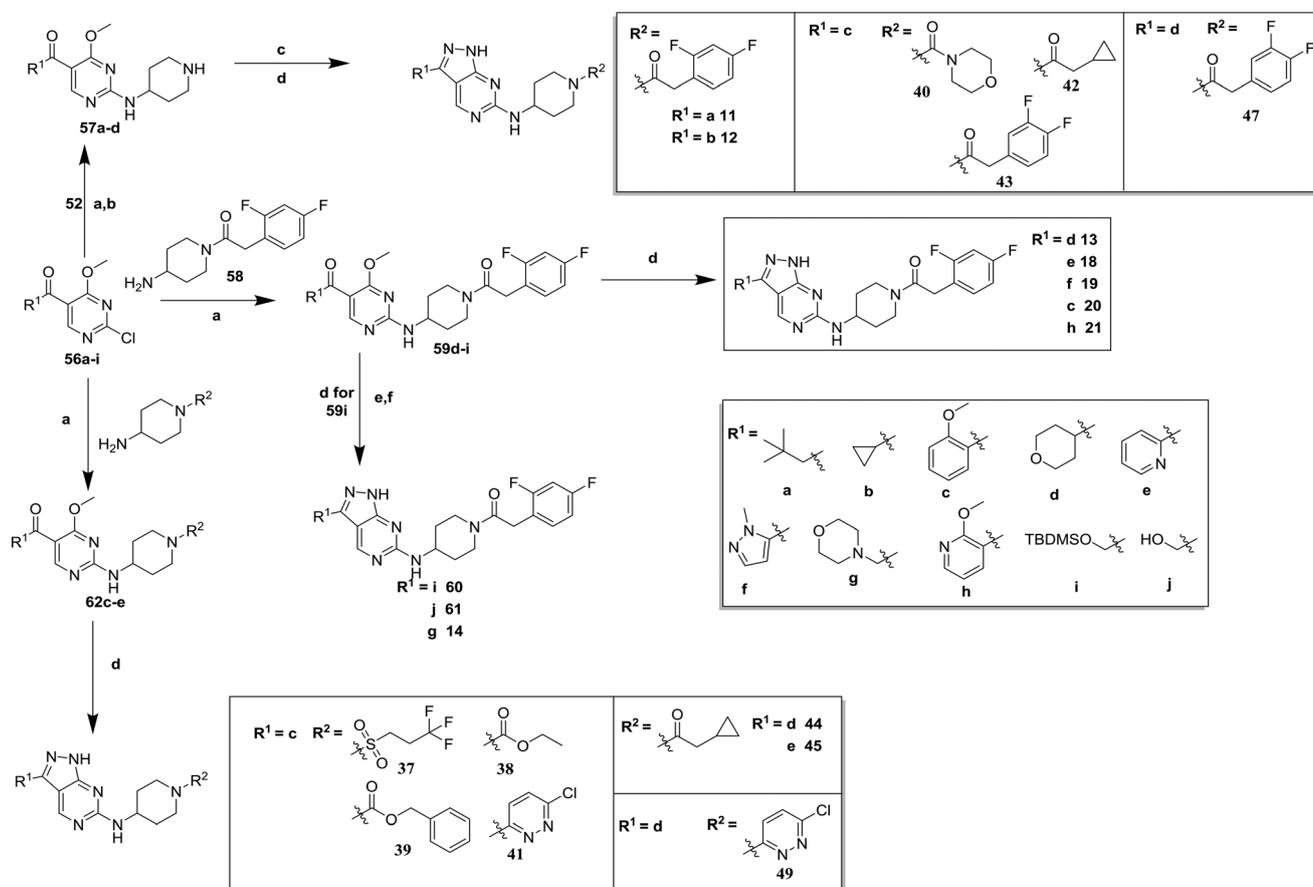
**Scheme 2** Synthesis of compounds 11–21, 37–45, 47 and 49. (a) DIPEA, butan-1-ol; (b) TFA, DCM, 47–83% (over 2 steps); (c) *R*<sup>2</sup>-COOH, TBTU, DIPEA, dimethylformamide (DMF); (d) hydrazine hydrate, butan-1-ol, 22–48% (over 2 steps); (e) tetra-*n*-butylammonium fluoride (TBAF), THF, 86%; (f) methanesulfonyl chloride (MsCl), DIPEA, acetonitrile (MeCN) then morpholine, 18%.
