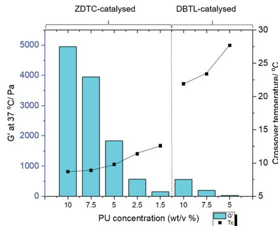
Fig. 3 Chart showing the storage moduli ( $G'$ , left vertical axis, bars) and crossover temperatures ( $T_c$ , right vertical axis, filled dots) of different concentrations of PU, whose syntheses are catalysed by either ZDTC or DBTL. At concentrations of  $<5.0$  wt/v%, the DBTL-catalysed PUs do not form gels below  $40$  °C.
