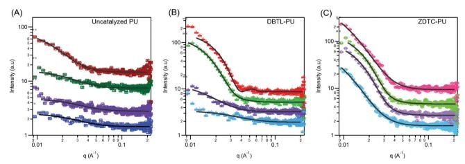
Fig. 6 Small-angle X-ray scattering patterns of 2 wt/v% aqueous solutions of (A) uncatalyzed PUs ( $\square$ ); (B) DBTL-catalysed PUs ( $\Delta$ ) and (C) ZDTC-catalysed PUs ( $\square$ ) at 4, 12, 25 and 37 °C. The solid black lines are model fits to the data. Curves are offset for clarity.
