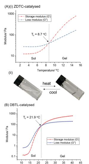
**Fig. 2** Oscillatory temperature sweep showing the changes in storage (G') and loss modulus (G'') as a function of temperature, as well as the gelation temperature of 10 wt% PU catalysed by (A) ZDTC and (B) DBTL. Figure (A)(ii) shows the reversible sol–gel transition of a transparent 10 wt/v% solution of ZDTC-catalysed PU in water.
