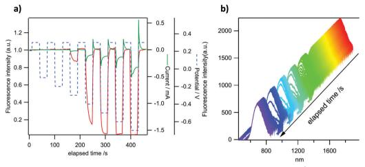
Fig. 10 Modulation of fluorescence intensity (red trace) and electrochemical current (green trace) of compounds  $8^{2+}$  (a) for potential steps of increasing amplitude (dashed blue trace). (b) Corresponding variation of emission spectra with time of compound  $8^{2+}$  for the same potential signal as in (a).
