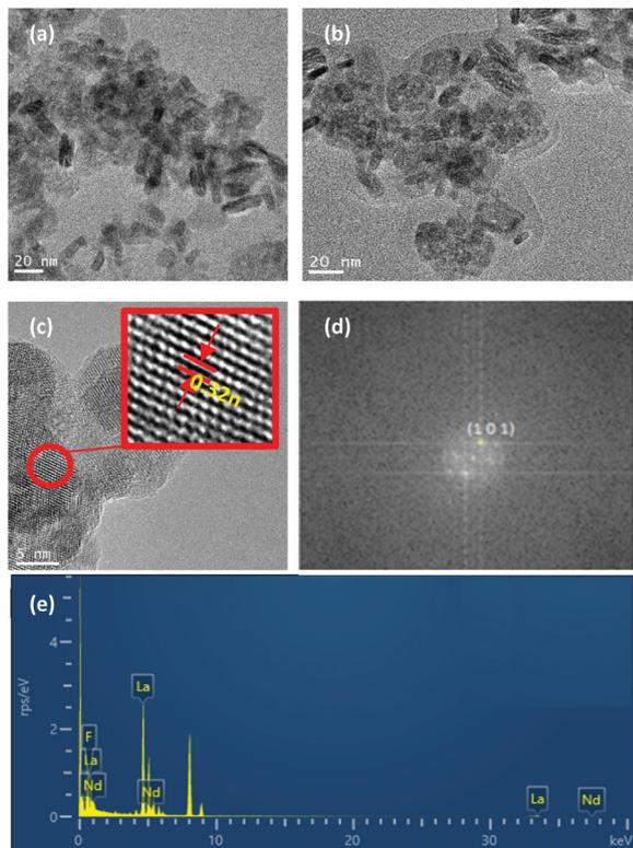
Fig. 3 HRTEM images of (a)  $\text{Nd}^{3+}$ - $\text{LaF}_3$ -0.04 M powder and (b)  $\text{Nd}^{3+}$ - $\text{LaF}_3$ -PVP(10)-0.25 M powder (c) single nanocrystal showing a lattice spacing of 0.325 nm for sample  $0.9\text{Nd}^{3+}$ - $\text{LaF}_3$ -0.25 M-PVP(10) (d) FFT pattern corresponding to (c) and (e) EDX analysis of the region.
