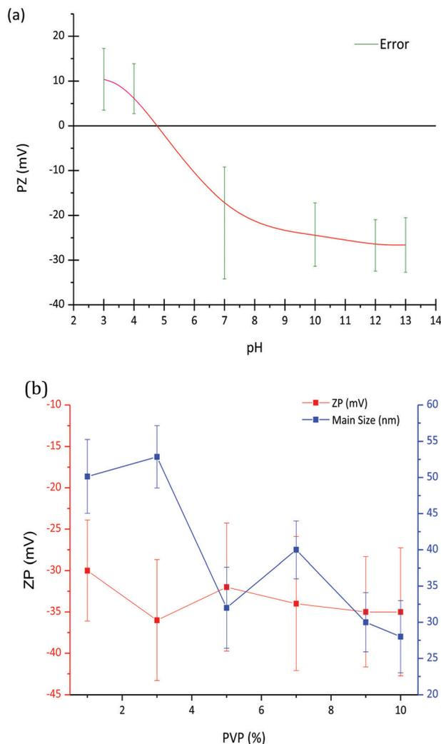
Fig. 1 (a) Variation of the ZP (mV) of LaF<sub>3</sub>-0.04 M nanoparticle suspensions as a function of pH and (b) variation of the zeta potential and particle size of LaF<sub>3</sub>-0.04 M nanoparticle suspensions at pH = 7 as a function of PVP wt%.
