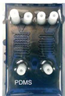
Fig. 2 PDMS templates with silica tubing guides. Adapted with permission from 71.
