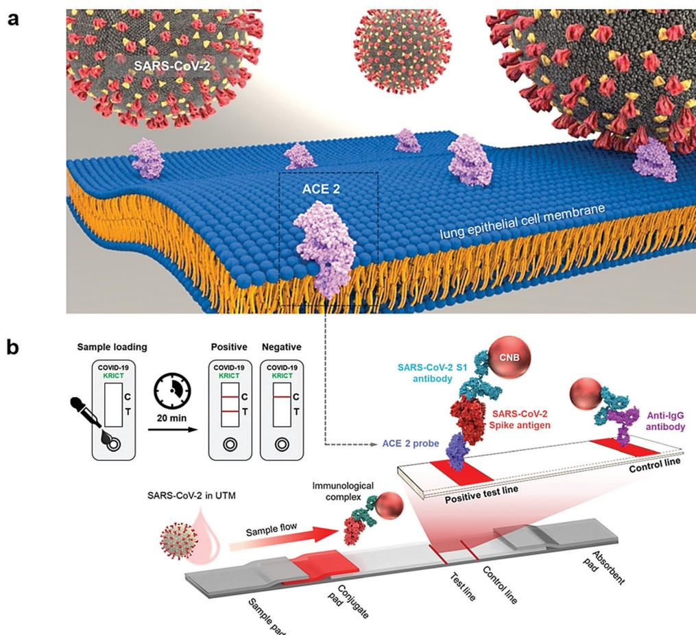
**Fig. 5** (a) The detection of SARS-CoV-2 spike 1 antigens using a cellular receptor (ACE2)-based LFIA. (b) The designed ACE2-based LFIA included a sample pad, conjugate pad, nitrocellulose membrane, and absorbent pad. The test line placed on the nitrocellulose membrane contains ACE2 for the detection of the SARS-CoV-2 spike antigen. The anti-IgG antibody was applied in the control line; and the detection result was achieved within 20 min. Reproduced with permission from ref. 44.
