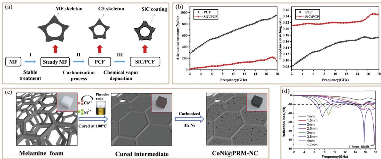
Fig. 5 (a) Three-step preparation process of the SiC/PCF composite.<sup>61</sup> (b) Impedance matching ratio and attenuation constant of PCF and SiC/PCF.<sup>61</sup> Reproduced with permission from ref. 61, Copyright © 2019, Elsevier. (c) Schematic illustration of CoNi@PRM-NC.<sup>120</sup> (d) Reflection loss curves of CoNi@PRM-NC.<sup>120</sup> Reproduced with permission from ref. 120, Copyright © 2019, Elsevier.
