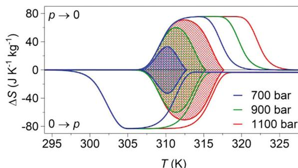
**Fig. 3** Pressure-driven isothermal changes in entropy on applying ( $0 \rightarrow p$ ) and removing ( $p \rightarrow 0$ ) selected hydrostatic pressures. Data shaded using different colours represent the reversible<sup>18</sup> barocaloric response at different pressures.
