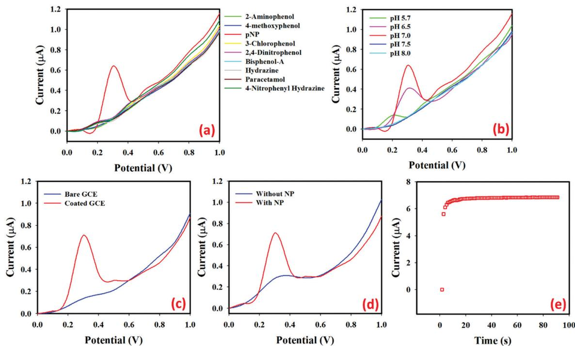
Fig. 3 *I*-*V* responses: (a) selectivity study using nine interferents, (b) pH variation; (c) bare GCE and MoO<sub>2</sub>·Fe<sub>3</sub>O<sub>4</sub>·CuO/GCE, and (d) without and with the presence of *p*-NP (1.0 μM; 25.0 μL), and (e) current variation with time for MoO<sub>2</sub>·Fe<sub>3</sub>O<sub>4</sub>·CuO/Nafion/GCE in 1.0 μM; 25.0 μL *p*-NP.
