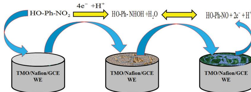
Scheme 1 The proposed mechanism in detection of *p*-NP by MoO<sub>2</sub>·Fe<sub>3</sub>O<sub>4</sub>·CuO/Nafion/GCE.
