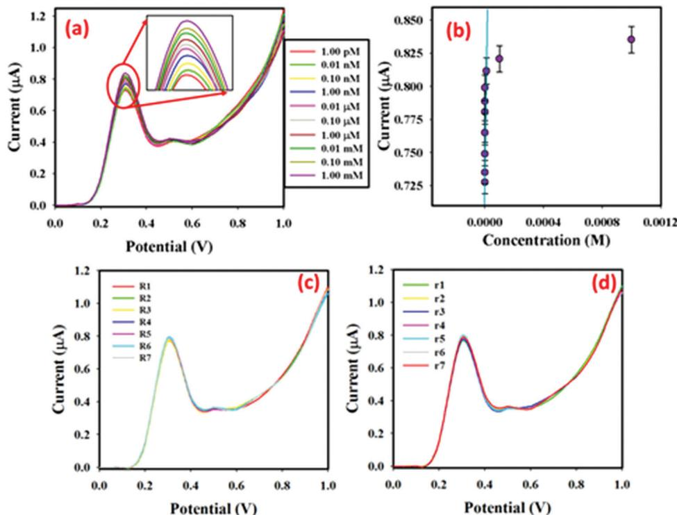
Fig. 4 (a) Current variations for different concentrations (1.0 pM to 1.0 mM) of aqueous *p*-NP in 0.0 to +1.0 V, (b) calibration plot of the MoO<sub>2</sub>-Fe<sub>3</sub>O<sub>4</sub>-CuO fabricated GCE at +0.3 V, (c) repeatability using different WEs (0.1 μM, 25.0 μL *p*-NP; 5.0 mL, 0.1 M PBS at pH 7.0), and (d) reproducibility using the same WE (0.1 μM, 25.0 μL *p*-NP; 5.0 mL, 0.1 M PBS at pH 7.0).
