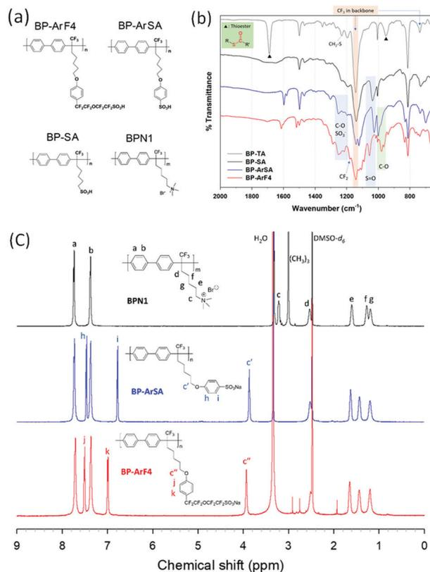
Fig. 1 Chemical structures and FT-IR spectra of the synthesized polymers. (a) Chemical structures of the polymers. (b) FT-IR spectra of the synthesized BP-TA (gray) and cation exchange polymers: **BP-SA** (black), **BP-ArSA** (blue), and **BP-ArF4** (red). (c)  $^1\text{H}$  NMR spectra (DMSO- $d_6$ ) of the synthesized polymers: **BPN1** (black), **BP-ArSA** (Na salt form, blue), and **BP-ArF4** (red; the peaks at 1.96, 2.78, and 2.94 ppm are from residual DMAc solvent from solvent casting).
