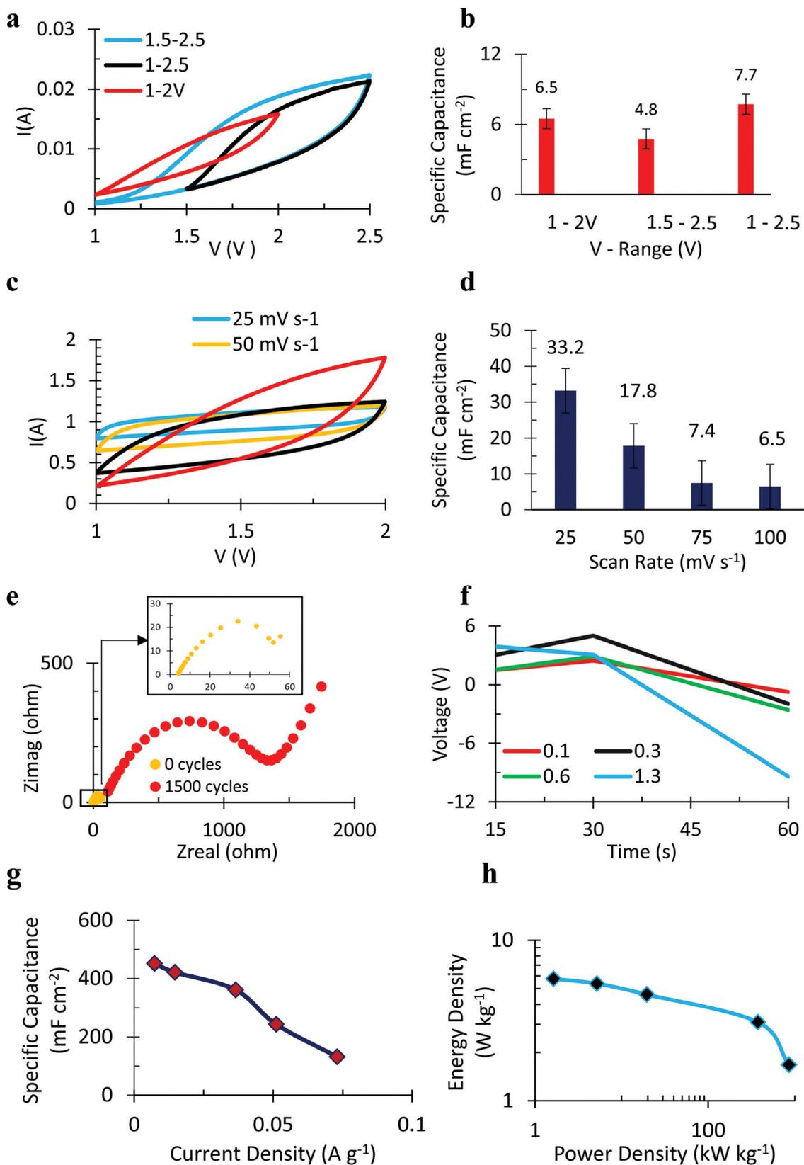
**Fig. 8** For the lig-Ni-CoWO<sub>4</sub>, CV plots for different potential windows (a) and at different scan rates (c); specific capacitance variation with voltage windows (b) and scan rates (d); Nyquist plot (e);  $V$  vs.  $T$  plot (f) at varying current density ( $A g^{-1}$ ); variation of specific capacitance with current density (g); and the Ragone plot (h).
