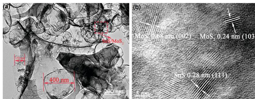
Fig. 4 TEM image (a) and high-resolution TEM (b) images of 3D SnS–MoS<sub>2</sub>@C.
