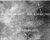
Fig. 4 TEM image (a) and high-resolution TEM (b) images of 3D  $SnS-MoS_2@C$ .
