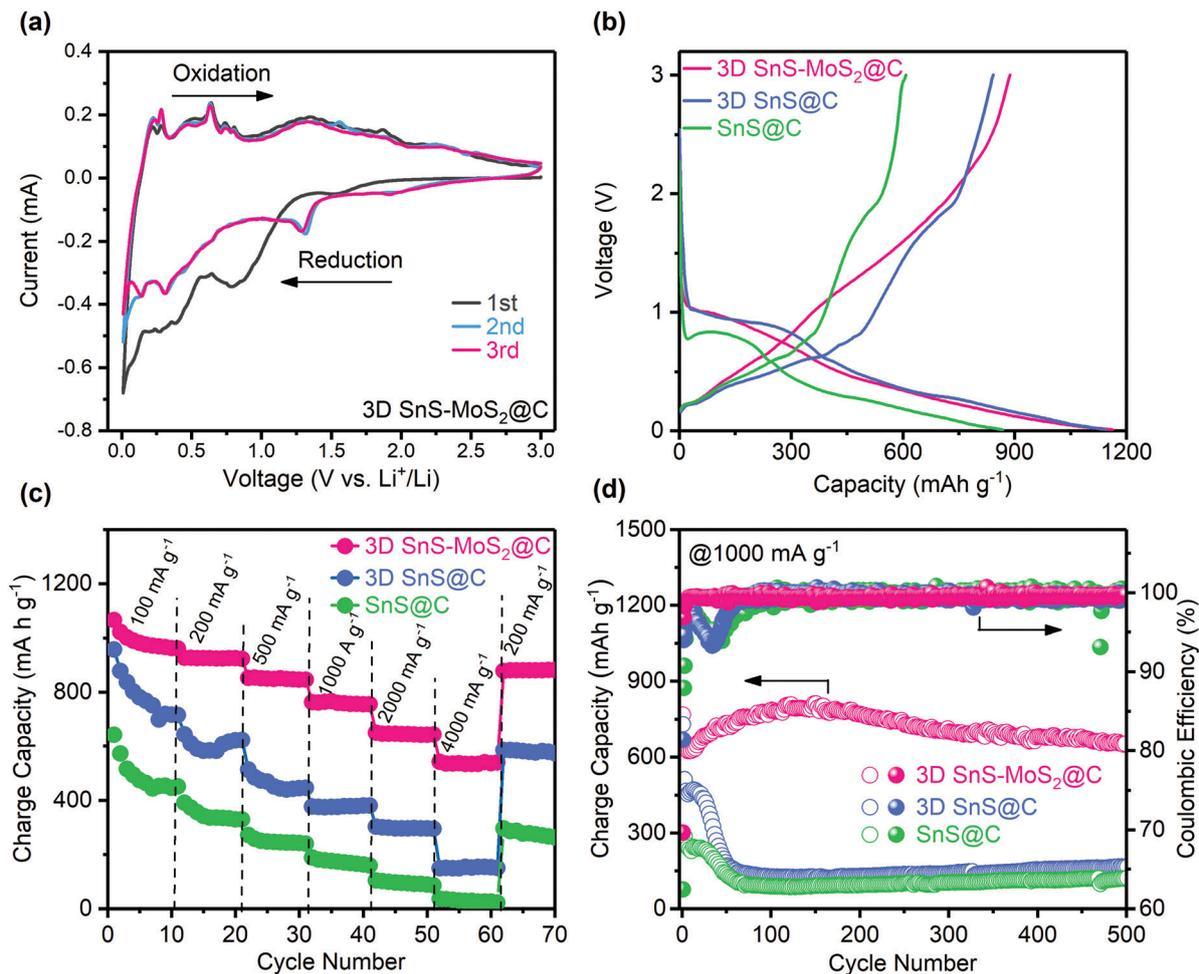
Fig. 6 Electrochemical characterization of the SnS-based electrodes. (a) Cyclic voltammetry (CV) of 3D SnS-MoS<sub>2</sub>@C at 0.1 mV s<sup>-1</sup>. (b) Voltage versus capacity curves of the three SnS-based electrodes at 200 mA g<sup>-1</sup>. Rate capability (c) and long-term cycling performance (d) of the three SnS-based electrodes.
