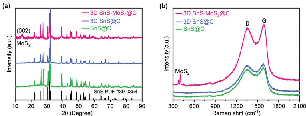
Fig. 3 XRD (a) and Raman (b) spectra of SnS@C, 3D SnS@C, and 3D SnS–MoS<sub>2</sub>@C. The powder diffraction file (PDF) standards for SnS is included for reference.
