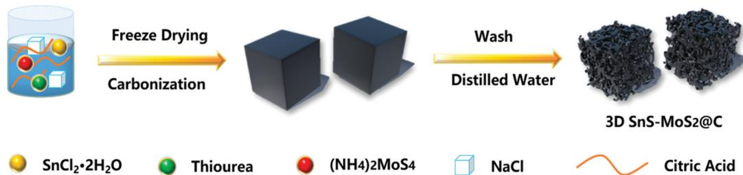
Fig. 1 Synthetic procedure for 3D SnS-MoS<sub>2</sub>@C.
