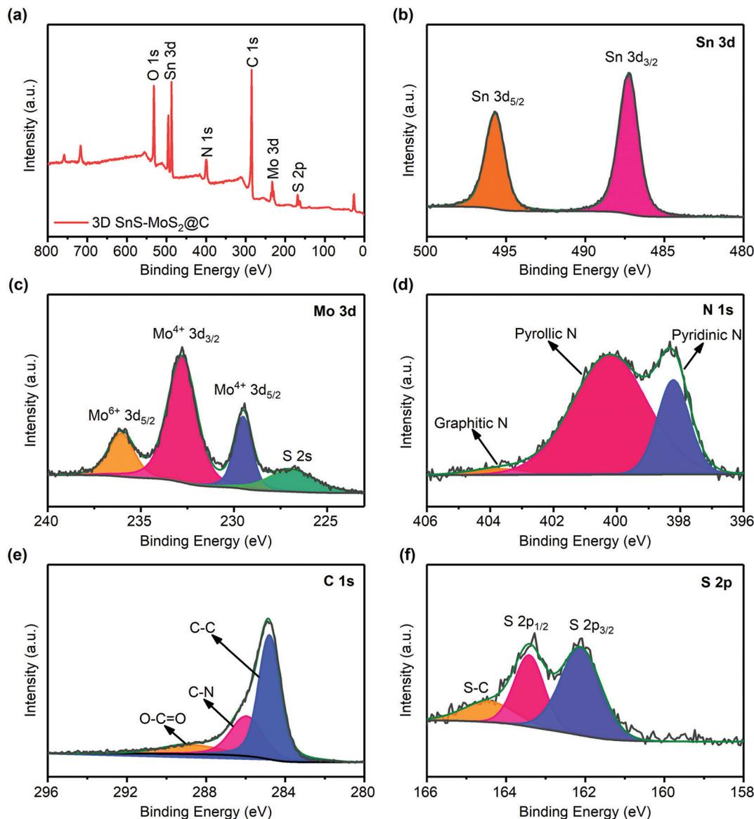
Fig. 5 (a) XPS survey spectrum of 3D SnS-MoS<sub>2</sub>@C. XPS spectra of Sn 3d (b), Mo 3d (c), N 1s (d), C 1s (e), and S 2p (f).
