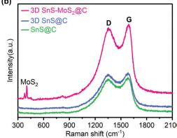
Fig. 3 XRD (a) and Raman (b) spectra of SnS@C, 3D SnS@C, and 3D SnS-MoS2@C. The powder diffraction file (PDF) standards for SnS is included for reference.
