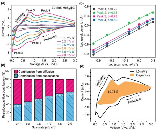
Fig. 7 (a) CV scans of the 3D SnS-MoS<sub>2</sub>@C anode at varying scan rates from 0.1 to 2.0 mV s<sup>-1</sup>. (b) Linear correlation between the logarithm of the peak currents and the logarithm of the scan rates. (c) Contribution of the pseudo-capacitive process at different scan rates depicted by bar charts. (d) Current contribution of the pseudo-capacitive process (orange area) during the CV tests at 1.0 mV s<sup>-1</sup>.
