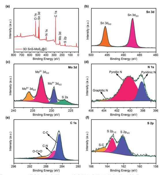
(a) XPS survey spectrum of 3D SnS-MoS<sub>2</sub>aC. XPS spectra of Sn 3d (b), Mo 3d (c), N 1s (d), C 1s (e), and S 2p (f).
