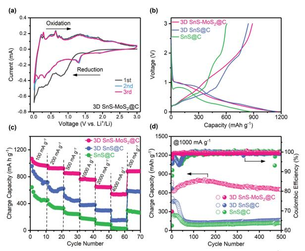
Fig. 6 Electrochemical characterization of the SnS-based electrodes. (a) Cyclic voltammetry (CV) of 3D SnS-MoS $_2$ @C at 0.1 mV s $^{-1}$ . (b) Voltage *versus* capacity curves of the three SnS-based electrodes at 200 mA g $^{-1}$ . Rate capability (c) and long-term cycling performance (d) of the three SnS-based electrodes.
