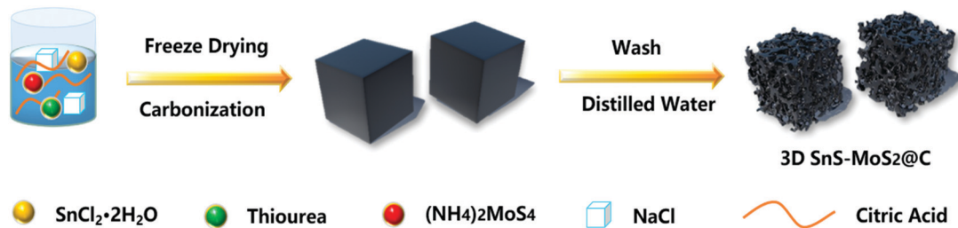
Fig. 1 Synthetic procedure for 3D SnS-MoS 2 @C.
