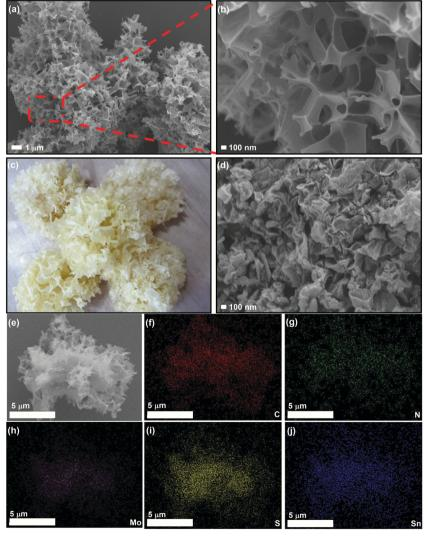
Fig. 2 (a) and (b) FESEM images of the as-prepared 3D SnS-MoS<sub>2</sub>@C. (c) Digital image of white fungus. (d) FESEM images of SnS@C and (e)-(j) EDS mapping (C, N, Mo, S, and Sn) images of the 3D SnS-MoS<sub>2</sub>.
