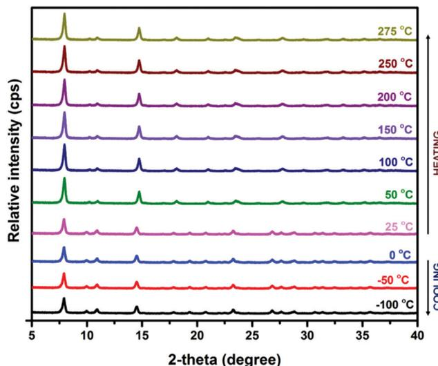
Fig. 2 Variable temperature PXRD patterns of Zn-CBS.
