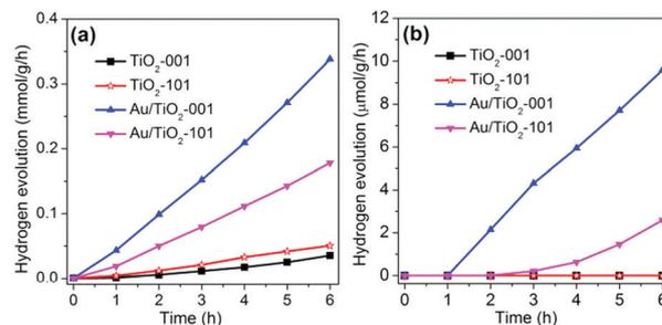
Fig. 4 The photocatalytic activity of hydrogen production rate for  $\text{TiO}_2$ -101,  $\text{Au/TiO}_2$ -101,  $\text{TiO}_2$ -001 and  $\text{Au/TiO}_2$ -001 samples under (a) simulated solar light or (b) visible light ( $\lambda \geq 420 \text{ nm}$ ) irradiation.
