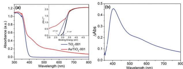
Fig. 2 (a) UV-vis DRS spectra of  $\text{TiO}_2$ -001 and  $\text{Au/TiO}_2$ -001 nanosheets. The inset graph shows the plots of  $[A(h\nu)]^{1/2}$  versus photon energy ( $h\nu$ ). (b) The subtracted DRS spectrum between  $\text{TiO}_2$ -001 and  $\text{Au/TiO}_2$ -001 nanosheets.
