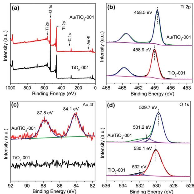
Fig. 3 (a) Typical XPS survey spectra of  $\text{TiO}_2$ -001 and  $\text{Au/TiO}_2$ -001 nanosheets. The high resolution XPS spectra of Ti 2p, Au 4f and O 1s (b, c and d, respectively) for the  $\text{TiO}_2$ -001 and  $\text{Au/TiO}_2$ -001 nanosheets.
