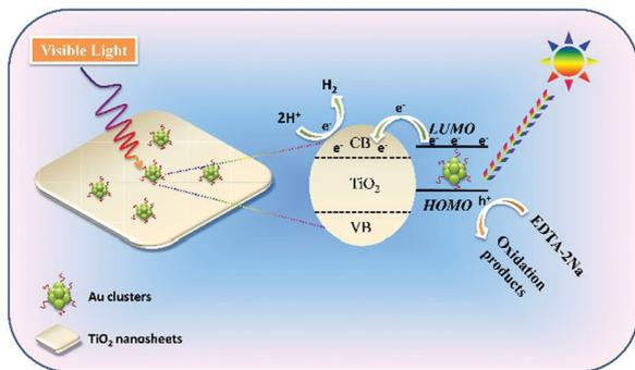
Fig. 5 Proposed mechanism of Au/TiO<sub>2</sub>-001 nanosheets for visible-light-induced photocatalytic hydrogen production.
