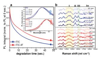
Fig. 2 AST on as-cast ITICs. In situ integrated PL intensity decay of as-cast ITIC (square) and ITIC-4F (circle) upon 633 nm laser excitation. Inset: Normalized PL spectra taken at different degradation times, for as-cast ITIC (upper panel) and ITIC-4F (lower panel) (a). In situ Raman spectra of as-cast ITIC (upper panel) and ITIC-4F (lower panel), corresponding to different degradation times upon 488 nm excitation (b).
