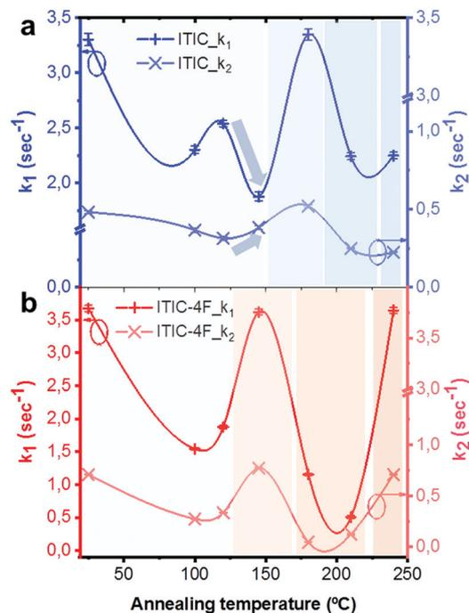
Fig. 9 Decay rates  $k_1$  and  $k_2$  extrapolated from the bi-exponential fitting of ITIC (a) and ITIC-4F (b) PL quenching profiles upon 633 nm laser irradiation, for different annealing temperatures of the materials.
