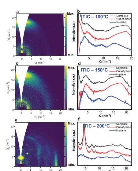
GIWAXS 2D patterns (a, c and e) and 1D in-plane and out-of-plane profiles (b, d and f) for ITIC annealed at different temperatures
