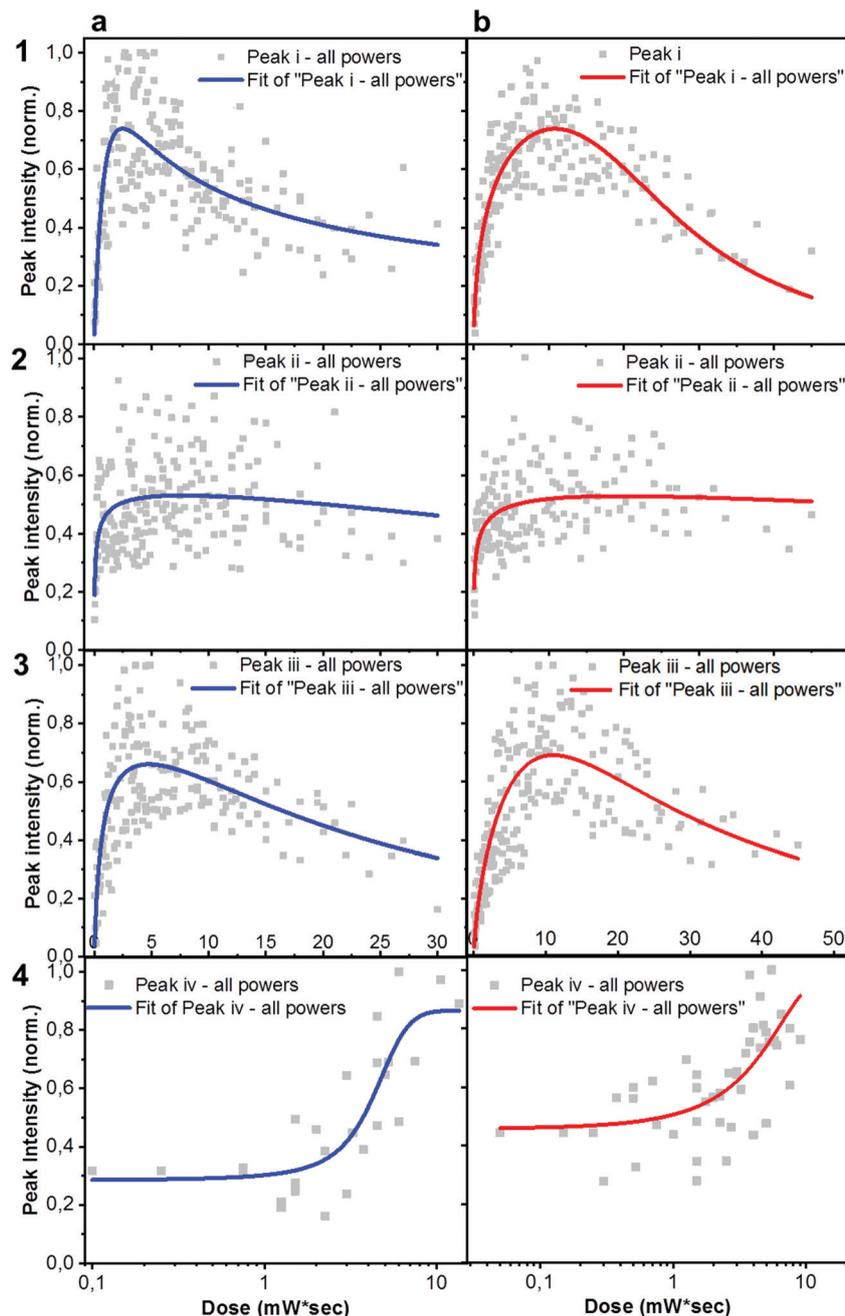
Fig. 3 Detailed Raman analysis of peaks evolution upon AST. Normalized integrated intensity of i ( $1450\text{ cm}^{-1}$ ), ii ( $1550\text{ cm}^{-1}$ ), iii ( $1600\text{ cm}^{-1}$ ) and iv ( $1750\text{ cm}^{-1}$ ) Raman peaks, extracted from Raman time series plots as a function of dose, for as-cast ITIC (column a) and ITIC-4F (column b) upon 488 nm excitation.
