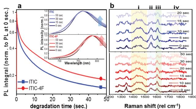
Fig. 2 AST on as-cast ITICs. *In situ* integrated PL intensity decay of as-cast ITIC (square) and ITIC-4F (circle) upon 633 nm laser excitation. Inset: Normalized PL spectra taken at different degradation times, for as-cast ITIC (upper panel) and ITIC-4F (lower panel) (a). *In situ* Raman spectra of as-cast ITIC (upper panel) and ITIC-4F (lower panel), corresponding to different degradation times upon 488 nm excitation (b).
