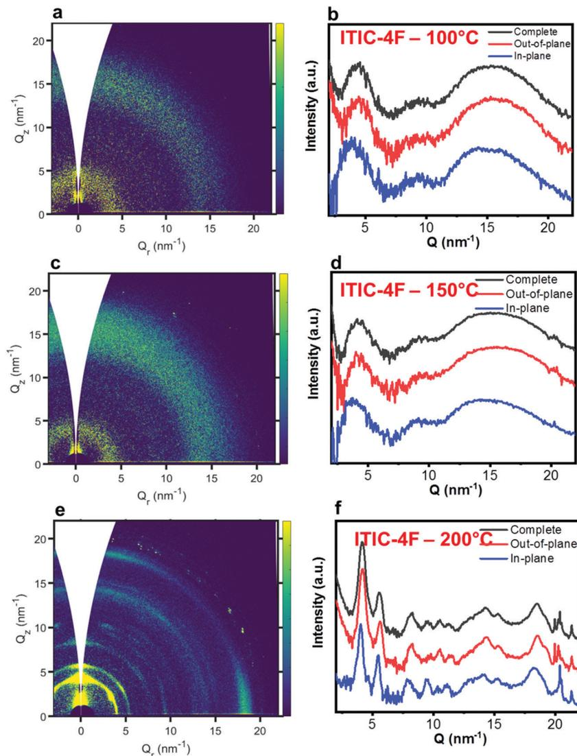
Fig. 7 GIWAXS 2D patterns (a, c and e) and 1D in-plane and out-of-plane profiles (b, d and f) for ITIC-4F annealed at different temperatures.
