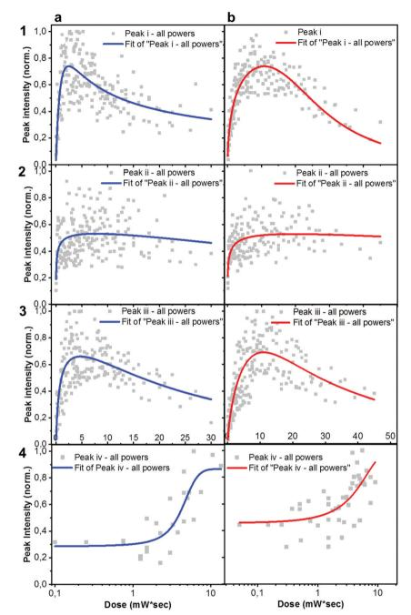
Fig. 3 Detailed Raman analysis of peaks evolution upon AST. Normalized integrated intensity of i ((1450) cm<sup>-1</sup>), ii ((1550) cm<sup>-1</sup>), iii ((1600) cm<sup>-1</sup>) and iv (\(\lambda 1750\rangle cm^{-1}\) Raman peaks, extracted from Raman time series plots as a function of dose, for as-cast ITIC (column a) and ITIC-4F (column b) upon 488 nm excitation.
