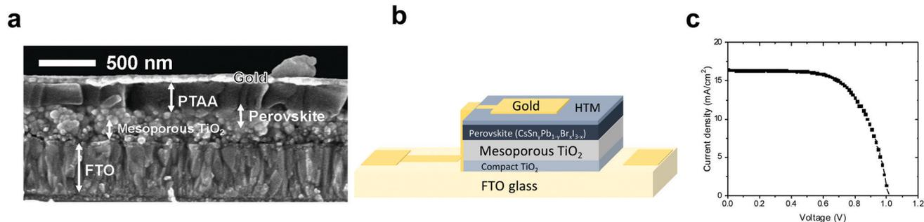
**Fig. 6** (a) Cross section SEM image of the PSC with a ratio of 80 : 20 ( $\text{CsSn}_{0.2}\text{Pb}_{0.8}|_{2.6}\text{Br}_{0.4}$ ) (Pb : Sn) and PTAA as the HTM. (b) Schematic illustration of the perovskite solar cell configuration used in this work. (c) *JV* curve of the champion cell presenting 12.7% efficiency, a FF of 64.2%, a  $J_{\text{sc}}$  of  $19.09 \text{ mA cm}^{-2}$  and a  $V_{\text{oc}}$  of 1 V.
