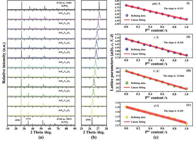
Fig. 2 (a) XRD patterns of the  $Sc(P_x,V_{1-x})O_4$  (0.0  $\leq x \leq 1$ ) solid solutions; (b) Enlarged XRD patterns within the range of 25–28°; (c) Experimentally calculated  $d_{hkl}$  values for the plane spacing (020) reflection (i), Rietveld refined lattice cell parameters a(b) (ii), c (iii), and cell volume (V) (iv) of the asobtained solid solutions as a function of  $P^{5+}$  (x) content.
