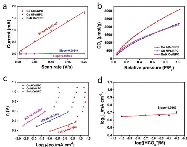
Fig. 5 Investigation of the catalytic mechanisms. (a) Charging current differences plotted as a function of the scan rates. The linear slope was used to estimate  $C_{dl}$  for Cu ACs/NPC, Cu NPs/NPC and bulk Cu/NPC. (b) CO<sub>2</sub> adsorption isotherms and (c) Tafel plots (overpotential vs.  $J_{CO}$ ) of the three catalysts. (d) Effect of HCO<sub>3</sub><sup>-</sup> concentration on the CO partial current density at a constant potential of  $-0.5$  V (vs. RHE) for Cu ACs/NPC.
