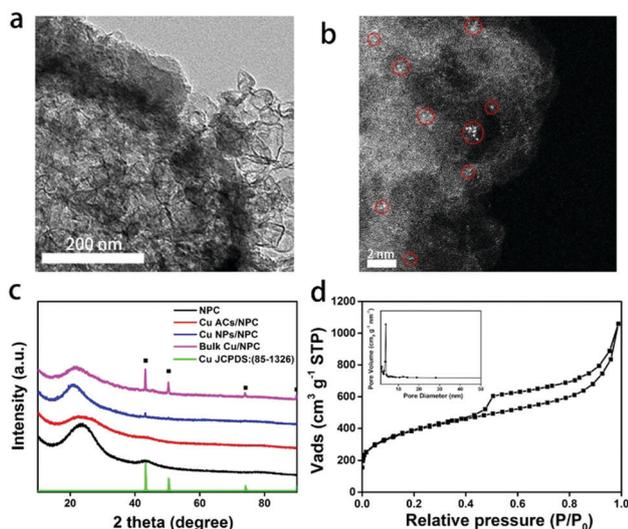
**Fig. 1** Structural characterization of Cu ACs/NPC. (a) TEM and (b) HAADF-STEM images of Cu ACs/NPC. (c) XRD patterns of NPC (black trace), Cu ACs/NPC (red trace), Cu NPs/NPC (blue trace), bulk Cu/NPC (pink trace) and standard Cu metal (green trace). (d)  $\text{N}_2$  adsorption-desorption isotherms and pore size distribution (inset) of Cu ACs/NPC.
