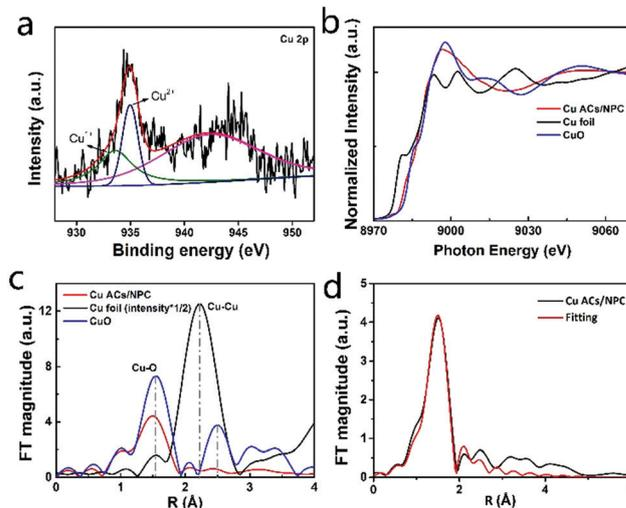
**Fig. 2** Electronic structural characterization of Cu ACs/NPC. (a) Cu 2p XPS spectra of Cu ACs/NPC. (b) Cu K-edge XAS spectra of Cu foil, CuO and Cu ACs/NPC. (c) Fourier transform curves of the EXAFS data of Cu foil, CuO and Cu ACs/NPC at Cu K-edge. (d) Fitting results of the EXAFS data for Cu ACs/NPC.
