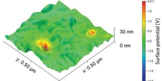
Fig. 10 Intermodulation electrostatic force microscopy of a spin coated 100 nm thick composite containing 3 wt% C8-coated ZnO nanoparticles measured with a DC bias of 2 V
