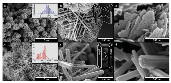
Fig. 1 Scanning electron micrographs of particles with different Zn/O surface terminations. Ball-shaped particles are shown in (a-c), where (c) shows the particles after 400 °C heat treatment. Rod-shaped particles are shown in (d-f), where (f) shows particles after 400 °C heat treatment. The insets in (a) and (d) show the size distributions of the particles, and the dominant crystal planes for ball- and rod-shaped particles are shown as insets in (b) and (e), respectively.
