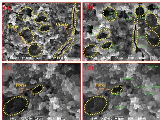
Fig. 4 SEM images (at different scales) showing that the morphology of the  $\text{Cu}_{0.8}\text{Zn}_{0.2}\text{Sb}_2\text{AAM}$  thin film possesses a highly porous rigid structure with few cracks and pores on the surface.
