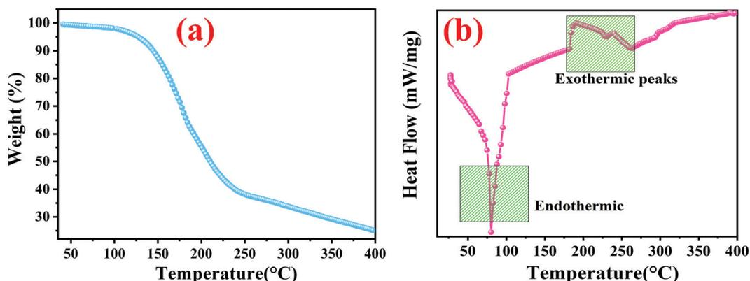
Fig. 10 (a) TGA and (b) DSC curves of  $\text{Cu}_{0.8}\text{Zn}_{0.2}\text{Sb}_2$  AAam under an argon atmosphere at a heating rate of 10 °C per minute.
