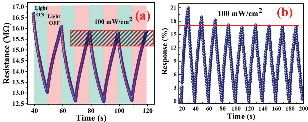
Fig. 12 (a and b) Photoconduction behaviour of the  $\text{Cu}_{0.8}\text{Zn}_{0.2}\text{Sb}_2\text{AAM}$  nanomaterial.
