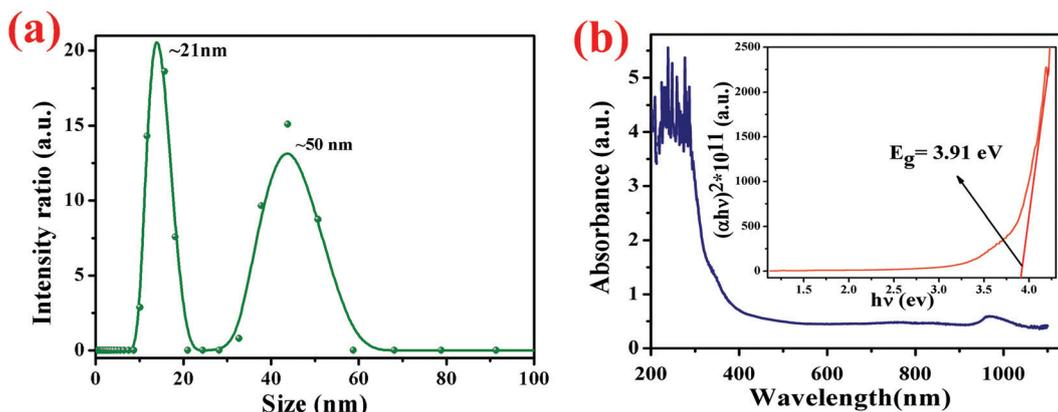
Fig. 8 (a) The particle size distribution curve shows that the peaks are divided into two major intensities; the first one is the peak of the particles at  $\sim 21$  nm with a second neighboring peak at 50 nm. (b) The optical absorbance spectrum of the fabricated film in the wavelength range of 190–1100 nm; the inset shows the Tauc plot.
