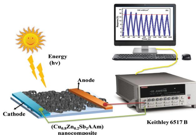
Fig. 2 A schematic diagram of the photoconduction set-up.
