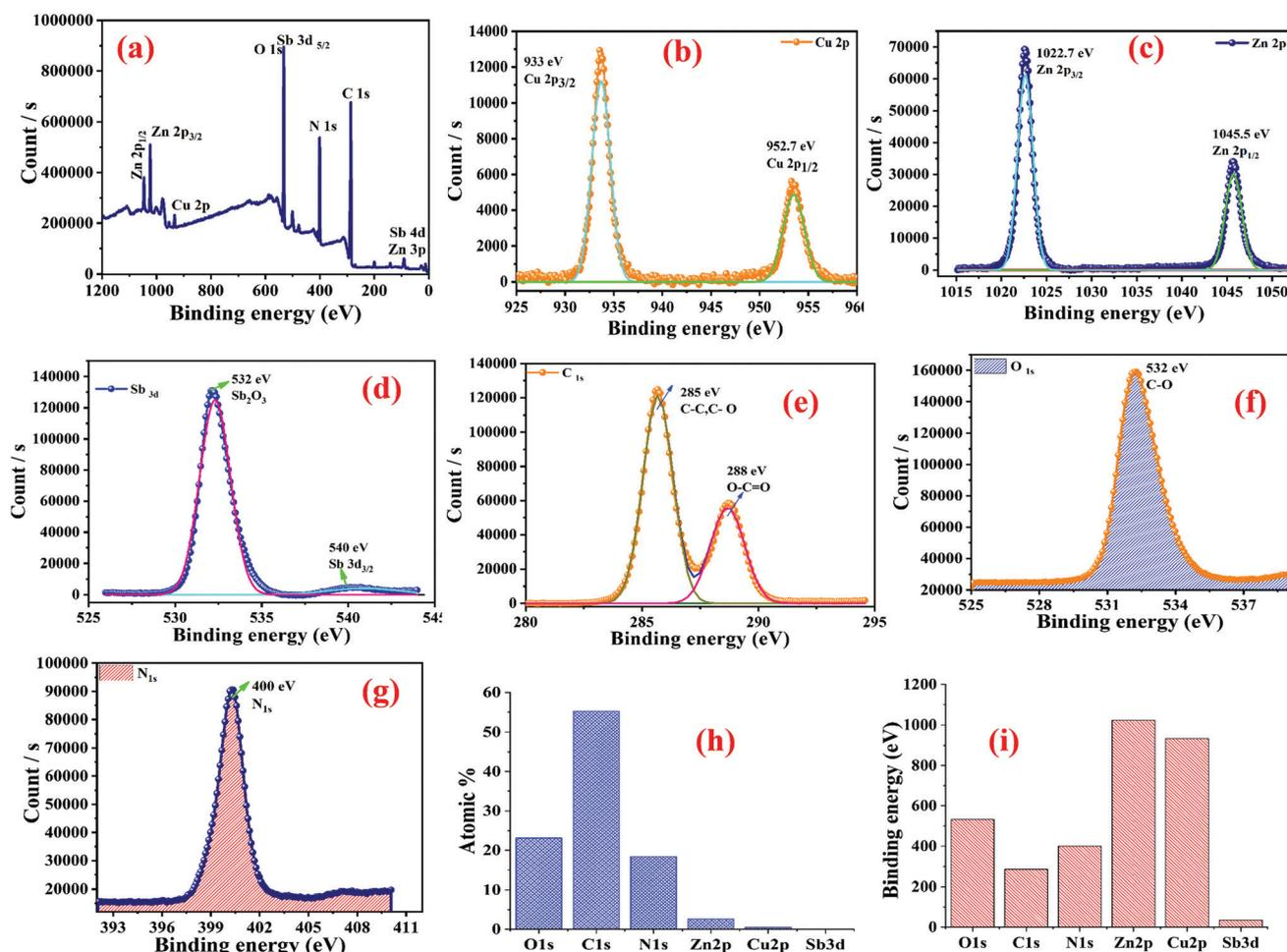
Fig. 11 XPS analysis of the  $Cu_{0.8}Zn_{0.2}Sb_2$  AAam nanocomposite: (a) survey; (b) copper (Cu 2p) element; (c) zinc (Zn 2p) element; (d) antimony (Sb 3d) element; (e) carbon (C 1s) element; (f) oxygen (O 1s) element; (g) nitrogen (N 1s) element; (h) atomic weight% values of the elements; and (i) a histogram showing the binding energies of the nanocomposites.
