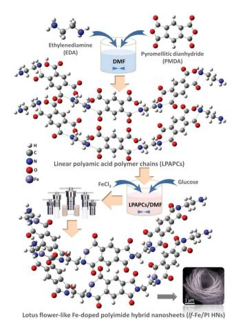
Fig. 1 Schematic illustration of the synthesis route of If-Fe/PI HNs.
