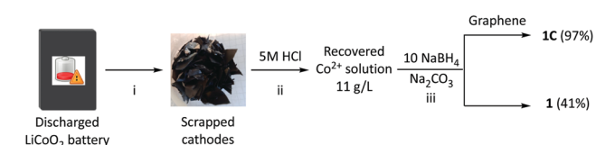
Scheme 2 Preparation sequence for 1 and 1C . (i) Manual dismantling and separation of cathode materials. (ii) Dissolution in 5 M \text{HCl} at 80 ^{\circ}\text{C} for 1 h. (iii) neutralisation and treatment with 10 eq. of \text{NaBH}_4 in ethanol, in the presence or absence of graphene.
