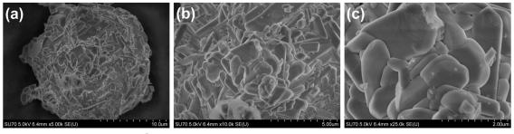
Fig. 2 SEM images of K<sub>2</sub>Bi(PO<sub>4</sub>)(MoO<sub>4</sub>):50%Sm<sup>3+</sup> powder at different magnifications
