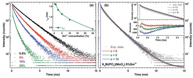
Fig. 6 (a) PL decay curves ( $\lambda_{ex}$  = 404 nm,  $\lambda_{em}$  = 598 nm) of K<sub>2</sub>Bi(PO<sub>4</sub>)(MoO<sub>4</sub>):Sm<sup>3+</sup> as a function of Sm<sup>3+</sup> concentration, inset shows average  $\tau$  values as a function of Sm3+ concentration. (b) Inokuti-Hirayama fit of K2Bi(PO4)(MoO4):5%Sm3+ sample PL decay curves. The upper inset shows enlarged part of the beginning of PL decay curve and the lower inset shows the respective residuals for fits with s = 6, 8, or 10.
