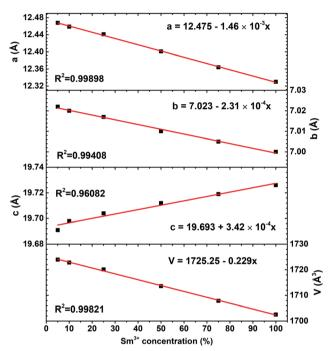
Fig. 3 Unit cell parameters of  $K_2Bi(PO_4)(MoO_4):Sm^{3+}$  as obtained from the Rietveld refinement.
