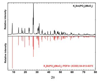
Fig. 1 XRD patterns of K<sub>2</sub>Sm(PO<sub>4</sub>)(MoO<sub>4</sub>) and K<sub>2</sub>Bi(PO<sub>4</sub>)(MoO<sub>4</sub>) reference.
