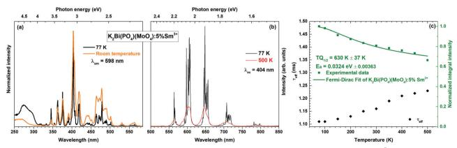
Fig. 5 Temperature dependent excitation ( $\lambda_{em}$  = 598 nm) and (b) emission ( $\lambda_{ex}$  = 404 nm) spectra of K<sub>2</sub>Bi(PO<sub>4</sub>)(MoO<sub>4</sub>):Sm<sup>3+</sup>, (c) calculation of TQ<sub>1/2</sub> value for the sample doped with 5% Sm<sup>3+</sup> from normalized emission intensity and  $\tau_{eff}$  values calculated from temperature dependent decay curves.
