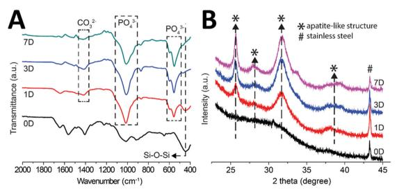
Fig. 8 (A) FTIR analysis of the multi-structured coatings before and after immersion in SBF for 1, 3, and 7 days, (B) XRD analysis of multi-structured coatings before and after immersion in SBF for 1, 3, and 7 days. PO
