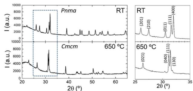
**Fig. 5** X-ray powder diffraction pattern of  $\text{Sn}_{1-\delta}\text{S}$  at room temperature and at 650 °C, showing the structural transition from the  $Pnma$  (room temperature) to the  $Cmcm$  space group at high temperatures. A magnification of the area enclosed by the dashed line is shown in the left part of the figure, including the Miller indices for the reflections.
