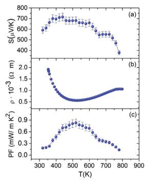
Fig. 7 Temperature dependence of the (a) Seebeck coefficient, (b) electrical resistivity and (c) power factor of  $Sn_{1-\delta}S$  synthesized using the microwave-hydrothermal method
