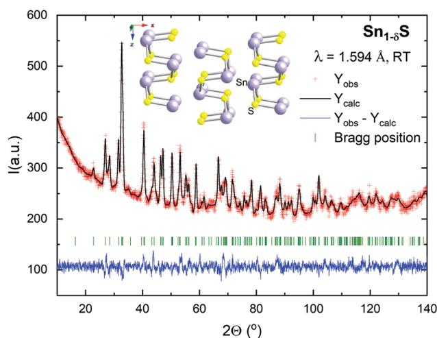
Fig. 2 Rietveld refinement from the powder neutron diffraction data of microwave-synthesized Sn<sub>1- $\delta$</sub> S: observed (red crosses), calculated (black line) and difference (blue line) profiles. The allowed Bragg positions are shown as green vertical marks. The crystalline structure obtained from the refined data is shown in the upper part of the figure (Sn atoms are represented in purple and S atoms in yellow).
