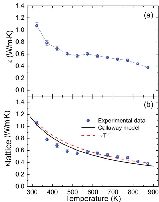
Fig. 10 Temperature dependence of the (a) total thermal conductivity and (b) lattice thermal conductivity of microwave-synthesized  $\text{Sn}_{1-x}\text{S}$ . The black solid line represents the data calculated using the Callaway model,<sup>76</sup> while the dotted line shows the  $\sim T^{-1}$  fit.
