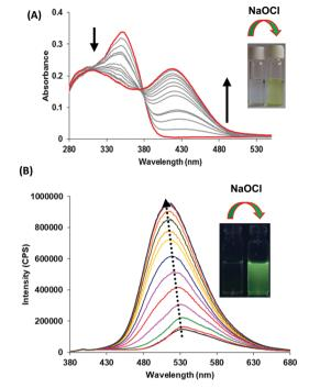
Fig. 1 (A) Absorption and (B) fluorescence emission spectra of probe 1 upon increasing concentration of hypochlorite (0-90 μM) in PBS/DMSO (8/2, v/v) mixture, pH = 7.4;  $\lambda_{ex}$  = 350 nm.
