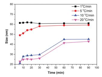
Fig. 4 Size vs. time curves at different heating rates.
