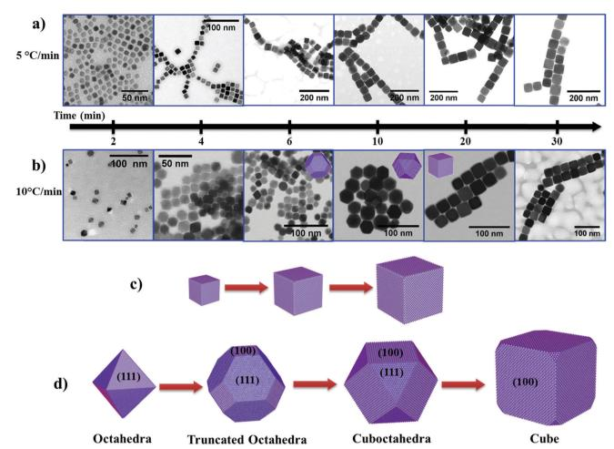
Fig. 3 BF STEM images showing the time dependent growth of  $Fe_3O_4$  nanocubes at two different heating rates: (a) 5 °C min<sup>-1</sup> and (b) 10 °C min<sup>-1</sup>. The reaction products were collected at different time intervals and analyzed with TEM. The proposed steps in the formation of nanocubes at (c) a slow heating rate (5 °C min<sup>-1</sup>) and (d) a faster heating rate (10 °C min<sup>-1</sup>). The image shown in panel (b) at 2 min is a TEM image.
