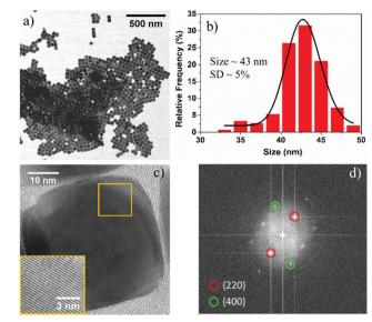
Fig. 1 (a) BF STEM image of  $Fe_3O_4$  nanocubes, (b) size distribution of nanocubes measured from the BF STEM image, (c) HRTEM image of a single crystalline nanocube and (d) fast Fourier transform (FFT) of the HRTEM image where the zone axis is [001]. The inset in panel (c) clearly shows the lattice fringes from the yellow square region of the NP.
