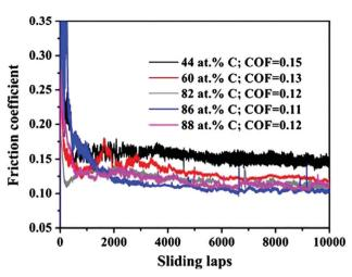
Fig. 9 Friction coefficient curves for coatings with 44–88 at% carbon concentrations against  $\mathrm{Si}_3\mathrm{N}_4$  balls as a function of sliding cycle. (Reproduced with permission from ref. 40.)
