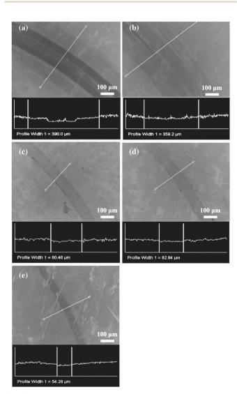
Fig. 10 SEM images of the wear tracks and profiles obtained from coatings with (a) 44, (b) 60, (c) 82, (d) 86 and (e) 88 at% carbon against  $\rm Si_3N_4$  balls after 10 000 laps. (Reproduced with permission from ref. 40.)
