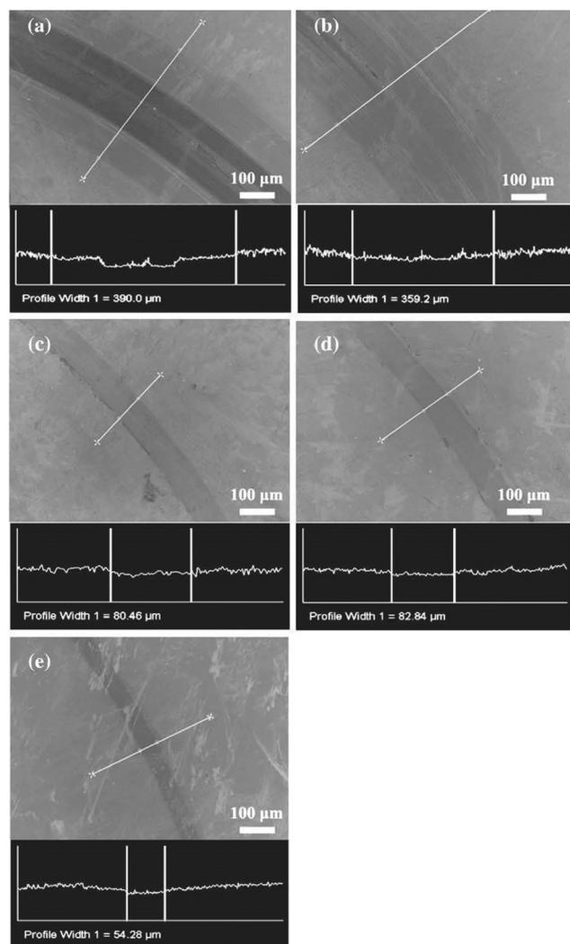
Fig. 10 SEM images of the wear tracks and profiles obtained from coatings with (a) 44, (b) 60, (c) 82, (d) 86 and (e) 88 at% carbon against  $\text{Si}_3\text{N}_4$  balls after 10 000 laps. (Reproduced with permission from ref. 40.)
