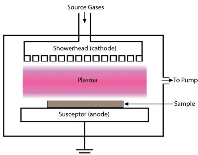
Fig. 4 Schematic illustration of a PECVD technique.
