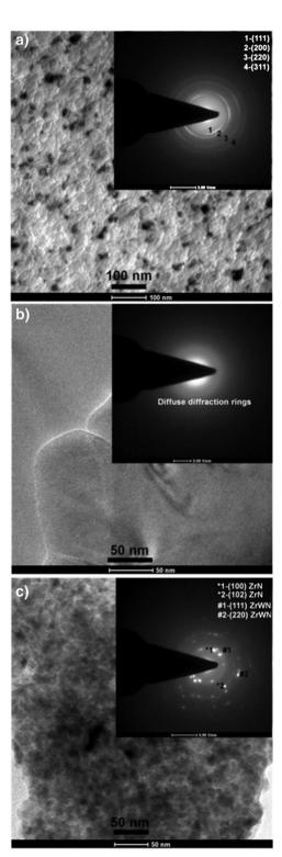
Fig. 6 Selected area diffraction patterns and bright field image topologies of (a) a single fcc phase (0.13 Pa), (b) an amorphous phase (0.27 Pa) and (c) a dual (fcc + hcp) phase (0.47 Pa). (Reprinted from ref. 116 with permission from Elsevier.)
