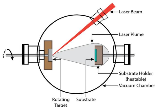
Fig. 3 A configuration for a PLD chamber.
