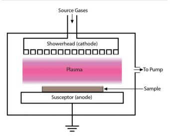
Fig. 4 Schematic illustration of a PECVD technique.
