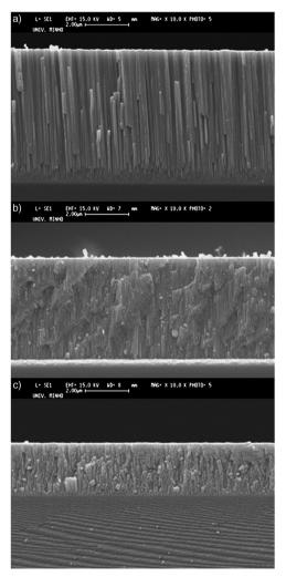
Fig. 8 Various morphologies of Zr-carbonitride films formed at Zr/(C + N) ratios of (a)  $\geq$  2.9, (b) 1.3 and (c)  $\leq$  0.7.
