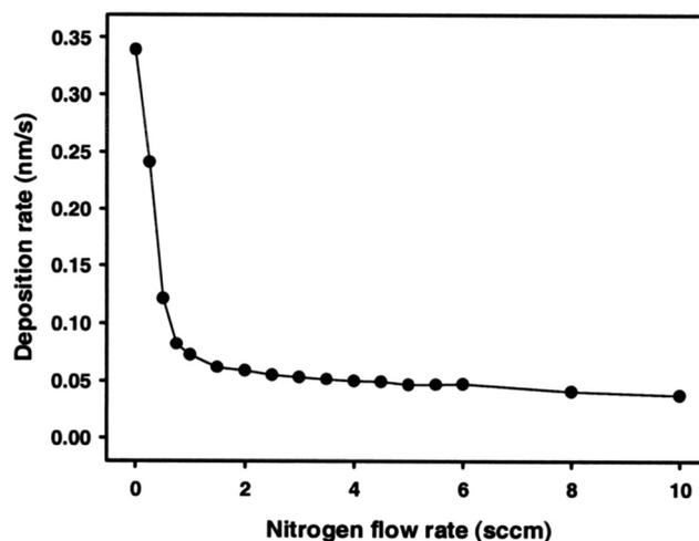
Fig. 5 Deposition rate of ZrN coatings decreases with increasing nitrogen flow rate during the RF sputtering process.<sup>148</sup> (Reproduced with permission from ref. 148.)
