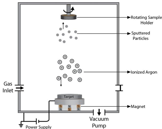
Fig. 1 Schematic illustration of a magnetron sputtering method.
