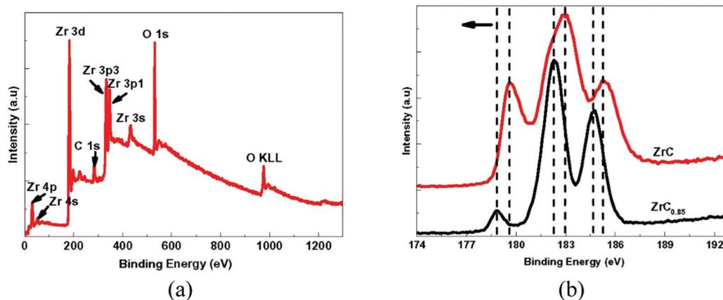
Fig. 18 XPS results obtained from ZrC coatings showing (a) a survey spectrum with peaks representing various energy levels. (b) Variation of intensity at core-levels in stoichiometric ZrC and non-stoichiometric ZrC<sub>0.85</sub> corresponding to Zr 3d. (Reproduced with permission from ref. 130.)
