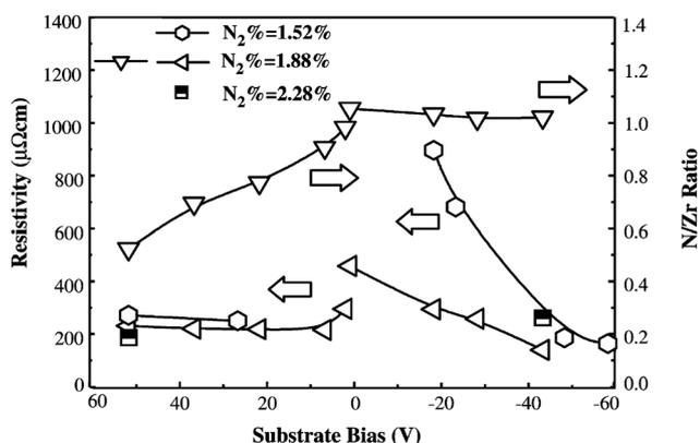
Fig. 14 Influence of the substrate bias (DC power = 150 W) on the resistivity and composition of ZrN<sub>x</sub> films. (Reproduced with permission from ref. 146.)
