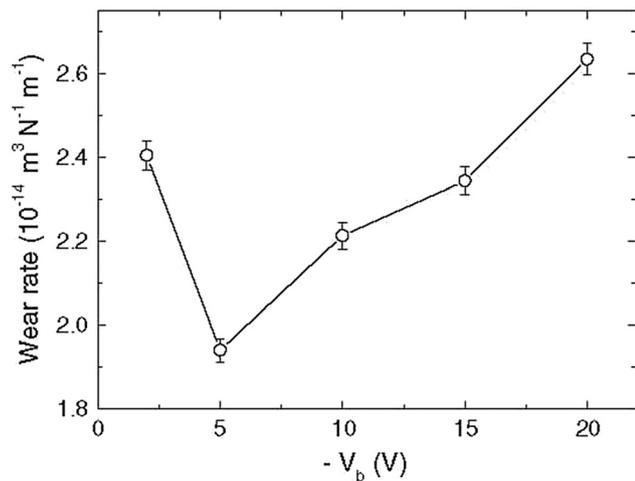
Fig. 15 Plot depicting the wear rate versus bias voltage. (Reproduced with permission from ref. 83.)
