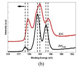
Fig. 18 XPS results obtained from ZrC coatings showing (a) a survey spectrum with peaks representing various energy levels. (b) Variation of intensity at core-levels in stoichiometric ZrC and non-stoichiometric ZrC<sub>0.85</sub> corresponding to Zr 3d. (Reproduced with permission from ref. 130.)
