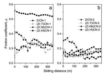
Fig. 17 Friction coefficients (μ) and sliding distances of ZrCN, (Zr,Ti)CN, (Zr,Hf)CN and (Zr,Nb)CN coatings: (a) low non-metal content and (b) high non-metal. (Reprinted from ref. 118 with permission from Elsevier.)
