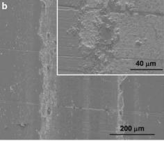
Fig. 16 SEM images of wear tracks formed on samples: (a) ZrN with 10 N load and (b) ZrN with 5 N load. Insets: High magnification images near the track edge. It can be seen that larger loads produced greater material removal. (Reproduced with permission from ref. 83.)
