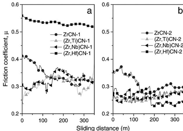
Fig. 17 Friction coefficients ( $\mu$ ) and sliding distances of ZrCN, (Zr,Ti)CN, (Zr,Hf)CN and (Zr,Nb)CN coatings: (a) low non-metal content and (b) high non-metal. (Reprinted from ref. 118 with permission from Elsevier.)
