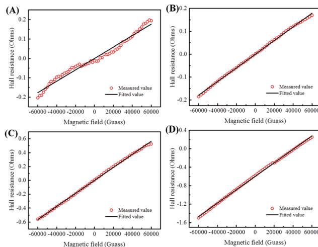
**Fig. 5** The Hall resistance value as a function of magnetic field for the optimized Te NWs thin piece (A and C) and that synthesized with  $N_2H_4 \cdot H_2O$  (B and D) before (A and B) and after (C and D) annealing at 350 °C for 3 h.
