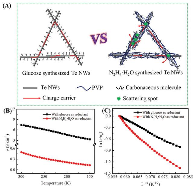
**Fig. 4** Schematic illustration of the highly conductive Te NWs synthesized with glucose (A). The dependence of electrical conductivity on temperature (B) and analysis of the temperature-dependence of the electrical conductivity with the 1D VRH model (C) of the optimized Te NWs thin piece and that synthesized with  $N_2H_4 \cdot H_2O$  before annealing.
