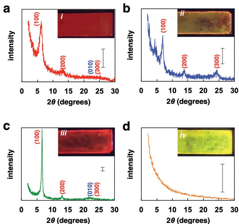
Fig. 4 XRD patterns of (a) **Film<sub>DCE</sub>**, (b) **Film<sub>MES</sub>**, (c) film after annealing then slow cooling, (d) film after annealing then rapid cooling. Scale bar: 100 counts.
