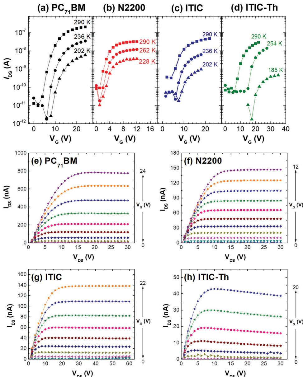
Fig. 4 Transfer and output characteristics of OTFTs using (a and e) **PC<sub>71</sub>BM**; (b and f) **N2200**; (c and g) **ITIC** and (d and h) **ITIC-Th** as the active layers.
