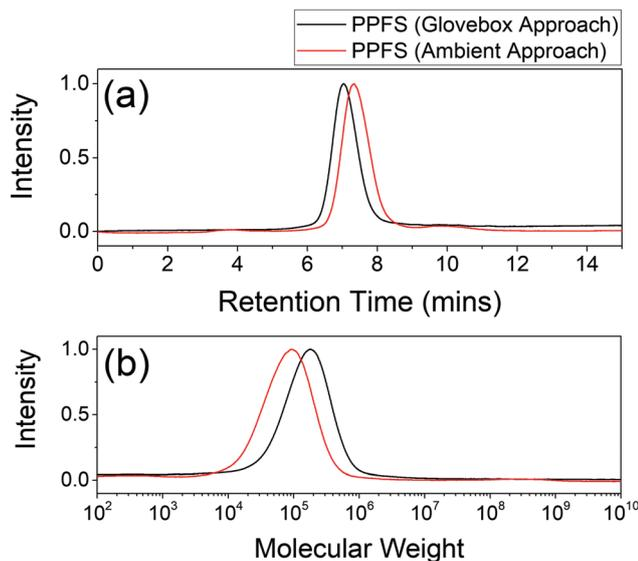
Fig. 1 (a) SEC chromatograms and (b) molecular weight distributions extracted from chromatography data of poly(2,3,4,5,6-pentafluorostyrene) (PPFS) via different synthetic conditions.
