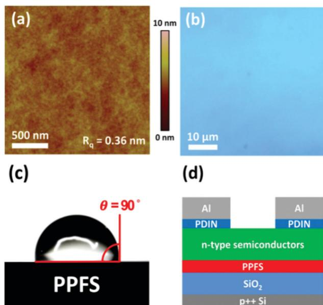
Fig. 3 (a)  $2\ \mu\text{m} \times 2\ \mu\text{m}$  atomic force microscopy and (b)  $50\ \mu\text{m} \times 50\ \mu\text{m}$  optical microscopy images of the **PPFS** film surface. (c) Water contact angle on the **PPFS**-coated  $\text{SiO}_2$  surface. (d) Schematic diagram of a bottom-gate-top-contact (BGTC) OTFT.
