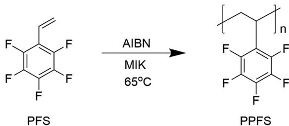
Scheme 1 General synthetic procedure of poly(2,3,4,5,6-pentafluorostyrene) (PPFS).
