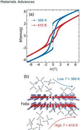
Fig. 2 Temperature effects on synthesis of molecular ferromagnet Fe(TCNE)<sub>v</sub>. (a) Magnetic hysteresis loops of Fe(TCNE)<sub>v</sub> at 50 K show that higher synthesis temperature improves the coercivity and homogeneity. (b) Reaction progress of FeSe and TCNE could be activated by heat energy. High enough synthesis temperature can improve the substitution reaction to obtain ferrimagnetic Fe(TCNE),
