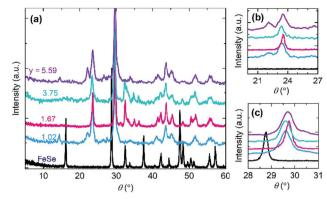
Fig. 3 X-Ray diffraction patterns of Fe(TCNE), synthesized at 410 K by a FeSe template. (a) XRD patterns of the whole range from 5° to 60° present the structure evolution from FeSe to  $Fe(TCNE)_{y}$  (y = 1.02, 1.67, 3.75 and 5.59). (b) Enlarged area of XRD patterns from 20° to 27°. (c) Enlarged area of XRD patterns from 28° to 31°
