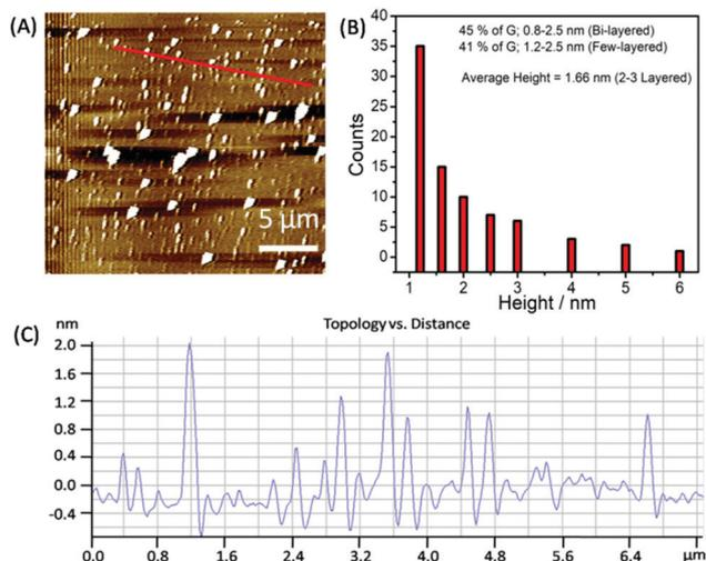
Fig. 4 AFM image of the exfoliated graphene flakes (A); the statistical analysis of the obtained height profile (B) and surface topology vs. the distance profile of exfoliated graphene flakes (C) corresponding to the red line shown in (A).
