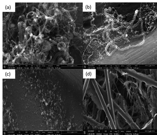
Fig. 2 Catalyst variation (Fe loading in  $\mu\text{g cm}^{-2}$  of carbon paper at 900  $^\circ\text{C}$ ): (a) 80  $\mu\text{g cm}^{-2}$ , (b) 90  $\mu\text{g cm}^{-2}$ , (c) 40  $\mu\text{g cm}^{-2}$  and (d) 20  $\mu\text{g cm}^{-2}$ .
