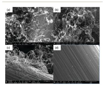
Fig. 3 Temperature variation (same Fe loading, 80  $\mu g$  cm<sup>-2</sup>): (a) 950 °C, (b) 900 °C, (c) 850 °C and (d) 800 °C.
