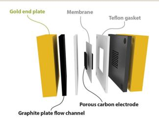
Fig. 1 Schematic representation of the in-house made flow cell with a serpentine flow channel (1.6 mm depth by 1.33 mm width).
