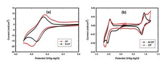
Fig. 5 CV comparison of CP and N-CP at the 0th cycle, in 0.1 M VOSO<sub>4</sub> in  $2 \text{ M} \text{ H}_2 \text{SO}_4$  at RT under  $\text{N}_2$  with a Ag-AgCl ref. electrode (183 mV/RHE) and high surface area graphite rod counter electrode, at a 10 mV s<sup>-1</sup> scan rate (a) anode, and (b) full window
