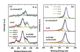
Fig. 8 (a) Deconvoluted XPS spectra of N 1s of the as received CP, N-CP and N-CP after 600 potential cycles on the anode, and (b) deconvoluted XPS spectra of C 1s of the as received CP, N-CP and N-CP after 600 potential cycles on the anode.
