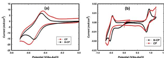
Fig. 5 CV comparison of CP and N-CP at the 0th cycle, in  $0.1 \text{ M VOSO}_4$  in  $2 \text{ M H}_2\text{SO}_4$  at RT under  $\text{N}_2$  with a  $\text{Ag-AgCl}$  ref. electrode ( $183 \text{ mV/RHE}$ ) and high surface area graphite rod counter electrode, at a  $10 \text{ mV s}^{-1}$  scan rate (a) anode, and (b) full window.
