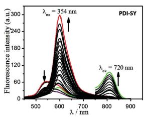
Fig. 3 Dual emission fluorescence spectra of **PDI-SY** as a function of the ClO $^-$  concentration, ([**PDI-SY**] = 2  $\mu$ M,  $\lambda_{ex}$  = 354 nm and 720 nm,  $V_{THF/H_2O}$  = 1:3, pH = 7.4, PBS buffer).
