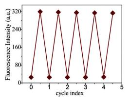
Fig. 7 Fluorescence intensity of **PDI-SY** at 600 nm ([**PDI-SY**] = 2  $\mu$ M,  $\lambda_{ex}$  = 354 nm, in  $V_{\text{THF/H}_2\text{O}}$  = 1:3, pH = 7.4, PBS buffer) upon addition of ClO (2 equiv.) and  $S^{2-}$  solution up to 5 cycles.
