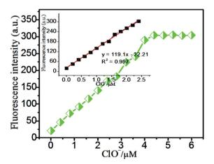
Fig. 4 Linear fitting curve of the probe **PDI-SY** with ClO $^-$ , ([**PDI-SY**] = 2  $\mu$ M, [ClO $^-$ ] = 2 equivalents,  $\lambda_{em}$  = 600 nm,  $V_{THF/H_2O}$  = 1:3).
