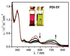
Fig. 2 Ratiometric absorption spectra of PDI-SY as a function of the ClO concentration, ([PDI-SY] = 2  $\mu$ M,  $V_{THF/H_2O}$  = 1:3, pH = 7.4, PBS buffer). The inset picture shows the color change of PDI-SY upon the addition of ClO-, L: PDI-SY, R: PDI-SY + CIO-.
