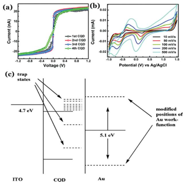
Fig. 6 (a)  $I$ - $V$  characteristic plots of PSS-Cdots recorded from different spots. (b) Cyclic voltammetry (CV) plot for aqueous PSS-Cdot dispersion at different scan rates. (c) Schematic representation corresponding to the band diagram of PSS-Cdot sandwiched between an indium tin oxide coated glass substrate (ITO) and a gold coated AFM tip (Au). Reprinted with permission from ref. 118. Copyright 2015 Royal Society of Chemistry.
