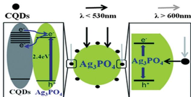
Fig. 5 Schematic representation corresponding to Cdote assisted improved photocatalytic activity of a Cdote/ $\text{Ag}_3\text{PO}_4$  complex. Reprinted with permission from ref. 115. Copyright 2012 Royal Society of Chemistry.
