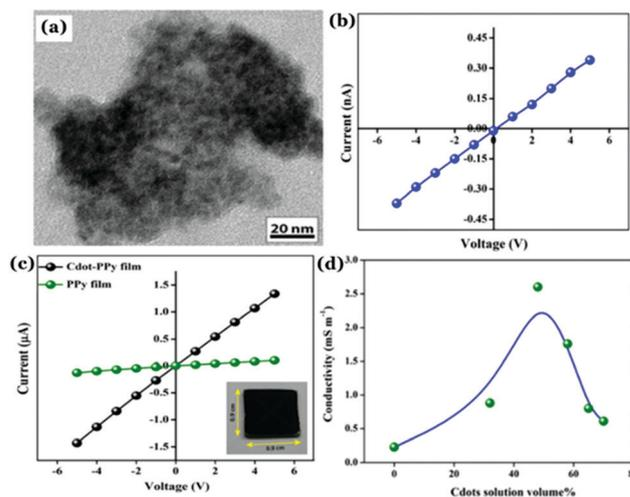
Fig. 7 (a) TEM image of the Cdot-PPy nanocomposite material. Plots of  $I$ - $V$  characteristics corresponding to (b) Cdot film and (b) Cdot-PPy and PPY films. (d) Change in the conductivity of the composite film due to the variation of Cdot content in the composite film. Reprinted with permission from ref. 119. Copyright 2016 American Chemical Society.
